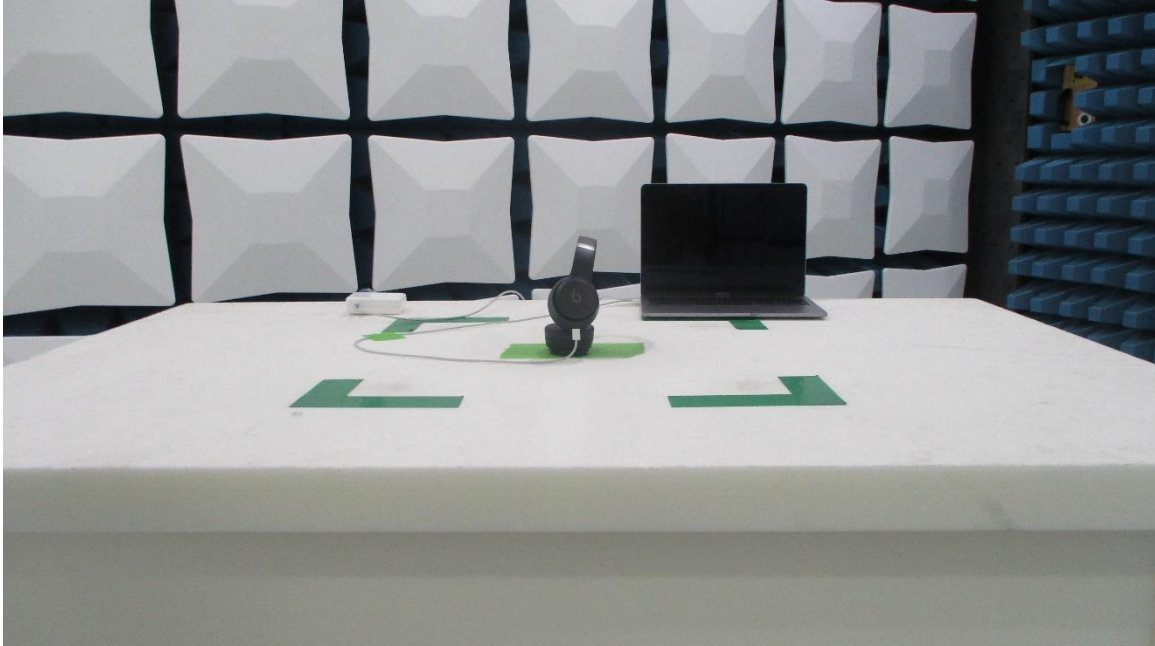
Figure 17: 30MHz-1GHz Test Setup (Front View)
