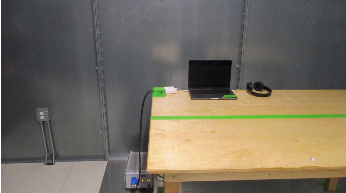
Figure 3: AC Line Conducted Emissions (Front View)
