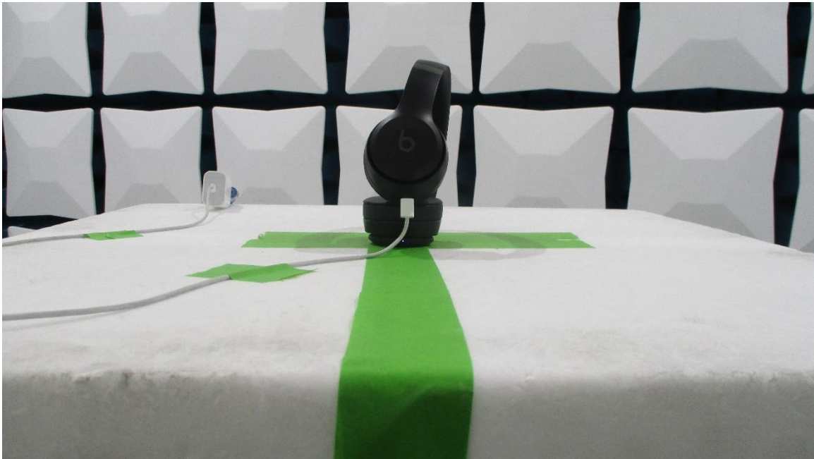
Figure 5: 1-18GHz Test Setup (Front View)
