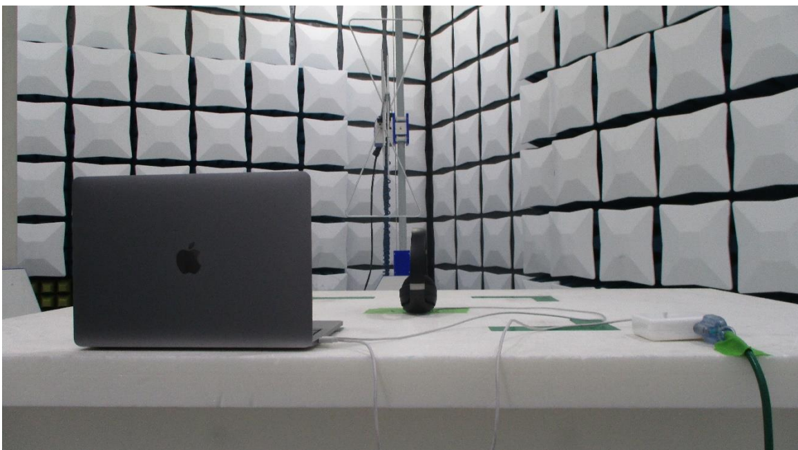
Figure 22: 30MHz-1GHz Test Setup (Rear View)
