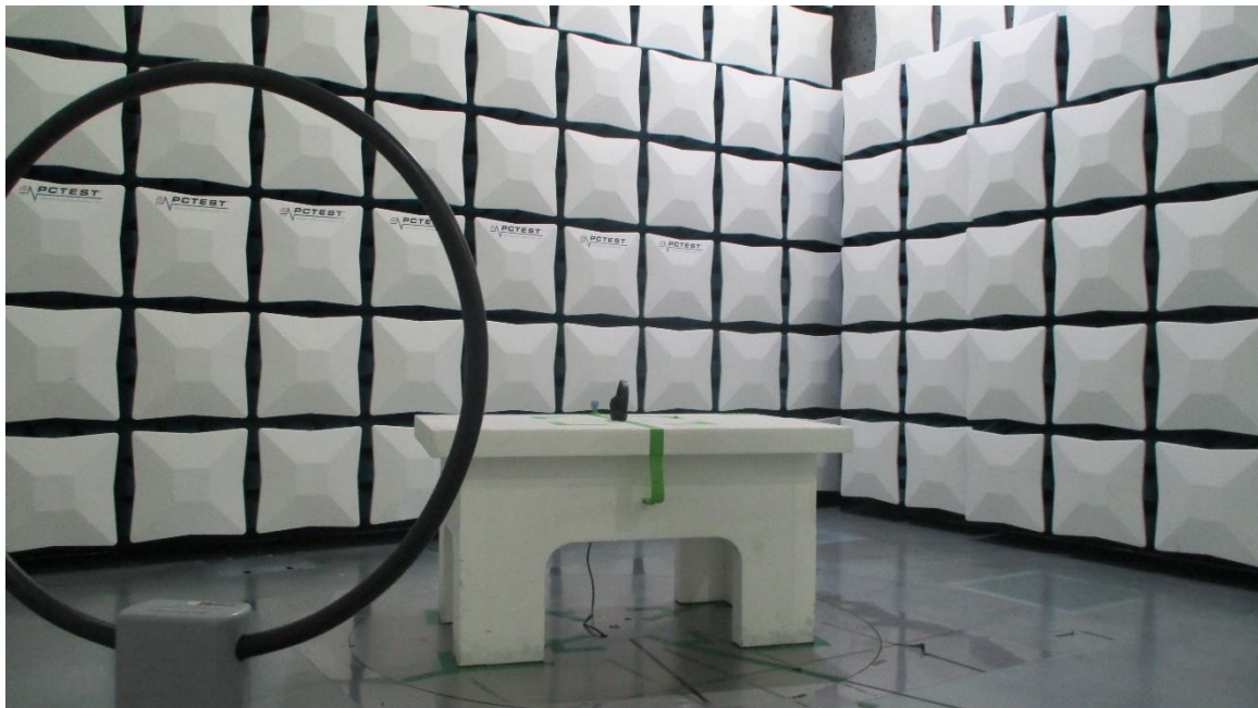
Figure 23: 9kHz-30MHz Test Setup (Front View)
