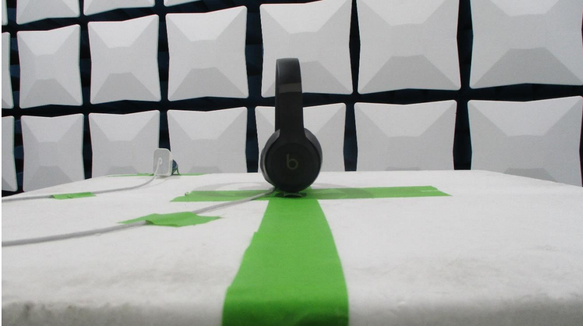
Figure 9: 1-18GHz Test Setup (Front View)
