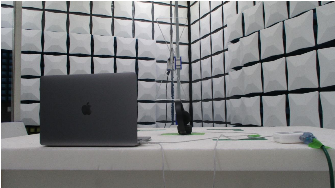
Figure 18: 30MHz-1GHz Test Setup (Rear View)
