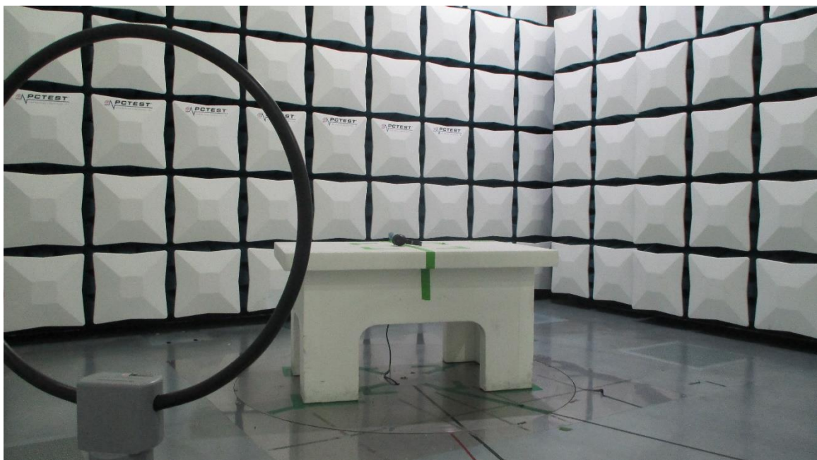
Figure 24: 9kHz-30MHz Test Setup (Front View)
