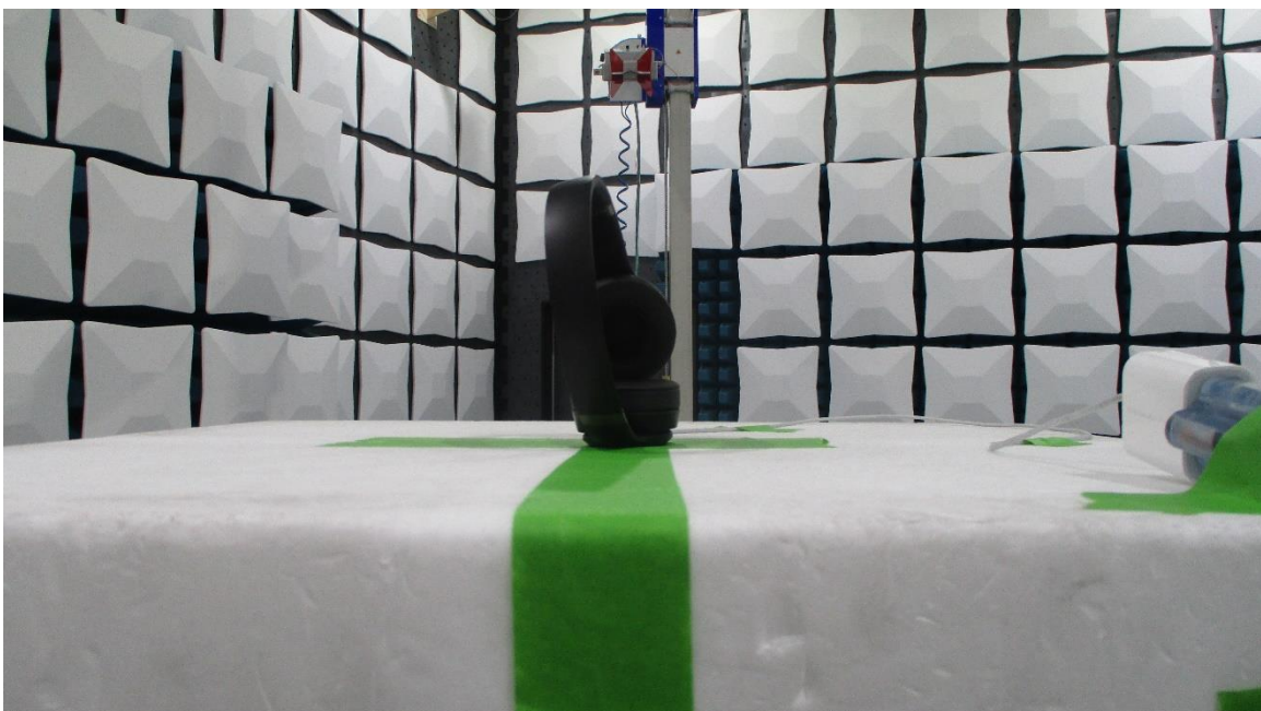
Figure 6: 1-18GHz Test Setup (Rear View)
