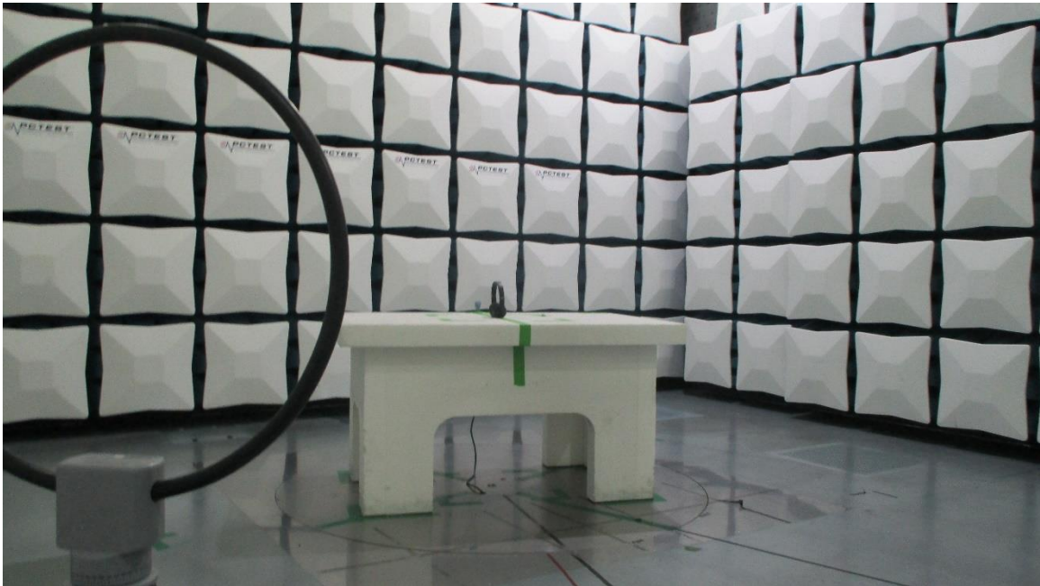
Figure 25: 9kHz-30MHz Test Setup (Front View)
