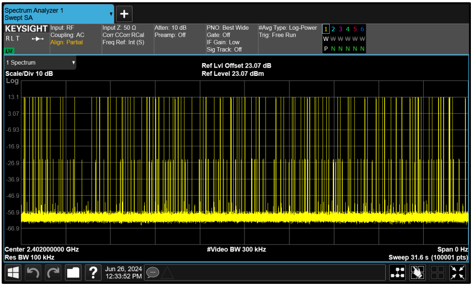
Figure 55 - GFSK - 2402 MHz Accumulated Transmit Time
