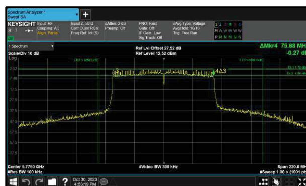
Figure 281 - 802.11ac VHT80 Maximum 6 dB EBW
