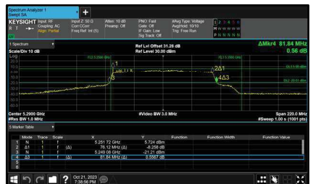
Figure 343 - 802.11ac VHT80 Maximum 99% OBW
