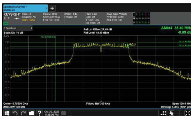
Figure 306 - 802.11n HT40 Minimum 6 dB EBW
