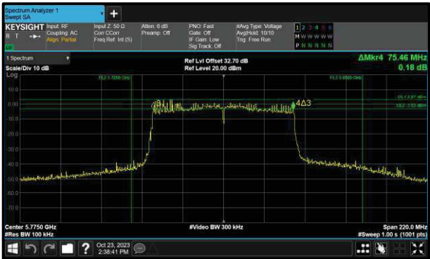
Figure 336 - 802.11ac VHT80 Minimum 6 dB EBW
