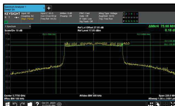
Figure 309 - 802.11ac VHT80 Maximum 6 dB EBW
