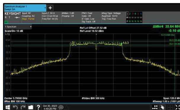
Figure 279 - 802.11n HT40 Maximum 6 dB EBW
