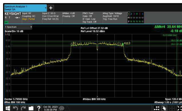
Figure 307 - 802.11n HT40 Maximum 6 dB EBW
