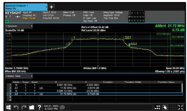
Figure 339 - Core 1 (B) 5180 MHz (CH36) 26 dB and 99% Bandwidth
