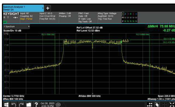
Figure 280 - 802.11ac VHT80 Minimum 6 dB EBW
