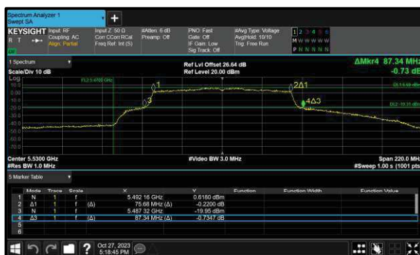
Figure 292 - 802.11ac VHT80 Minimum 99% OBW
