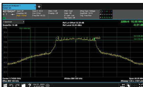
Figure 332 - 802.11ac VHT20 Minimum 6 dB EBW
