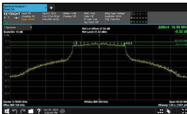
Figure 304 - 802.11n HT20 Minimum 6 dB EBW
