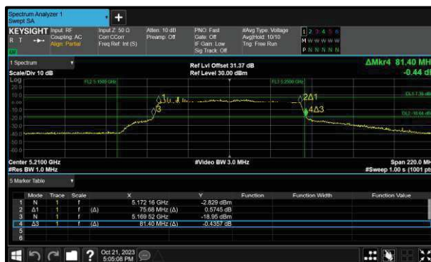
Figure 342 - 802.11ac VHT80 Minimum 99% OBW
