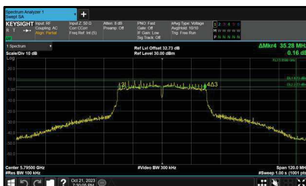
Figure 334 - 802.11ac VHT40 Minimum 6 dB EBW
