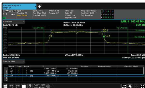
Figure 294 - 802.11ac VHT160 Minimum 99% OBW
