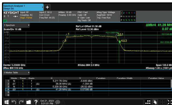
Figure 340 - 802.11ac VHT40 Minimum 99% OBW
