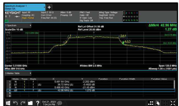
Figure 341 - 802.11ac VHT40 Maximum 99% OBW
