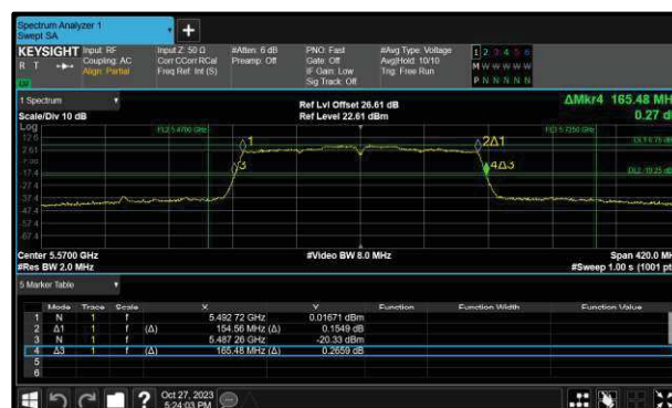
Figure 295 - 802.11ac VHT160 Maximum 99% OBW
