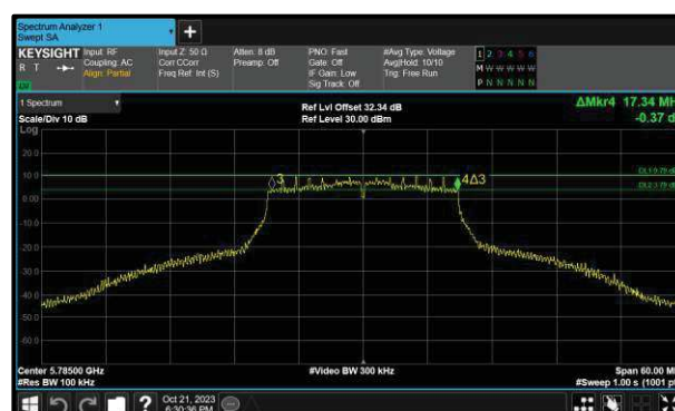
Figure 333 - 802.11ac VHT20 Maximum 6 dB EBW
