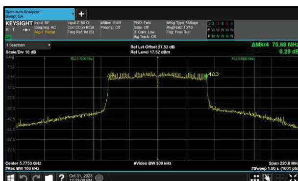
Figure 308 - 802.11ac VHT80 Minimum 6 dB EBW
