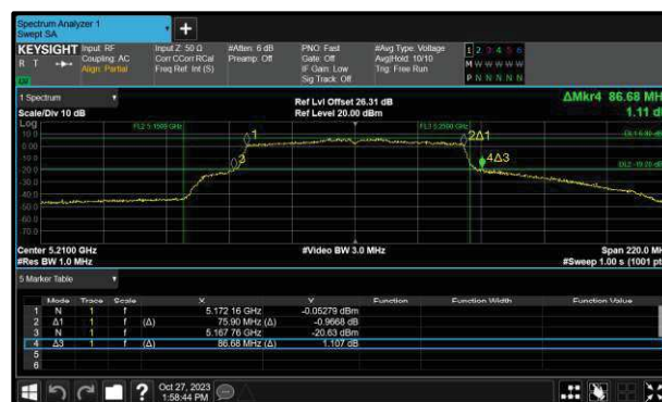
Figure 293 - 802.11ac VHT80 Maximum 99% OBW
