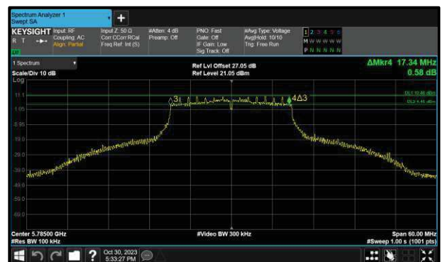
Figure 305 - 802.11n HT20 Maximum 6 dB EBW
