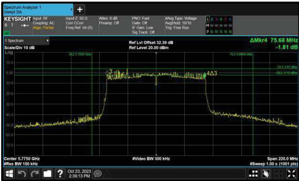
Figure 337 - 802.11ac VHT80 Maximum 6 dB EBW
