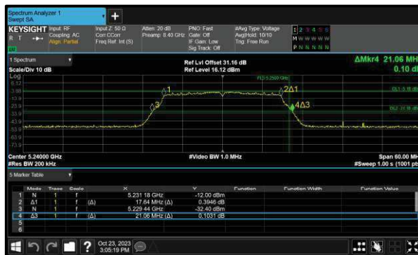
Figure 338 - Core 0 (A) 5180 MHz (CH36) 26 dB and 99% Bandwidth
