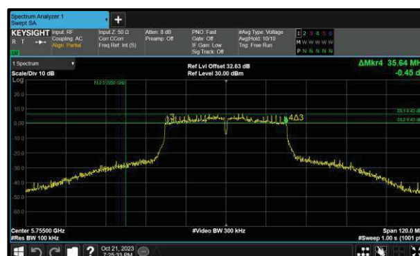
Figure 335 - 802.11ac VHT40 Maximum 6 dB EBW
