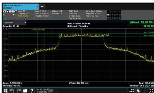
Figure 278 - 802.11n HT40 Minimum 6 dB EBW
