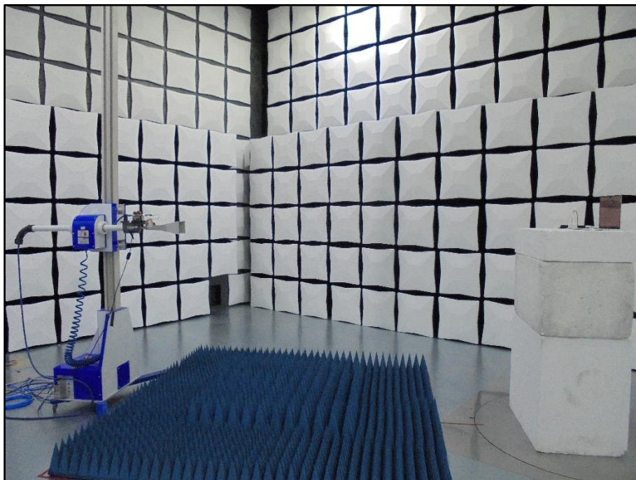
Figure 4 Radiated Disturbance - Above 1 GHz
