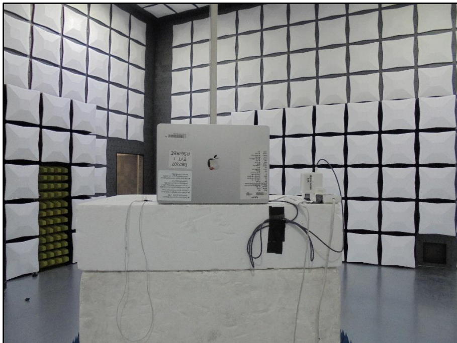
Figure 2 Radiated Disturbance - Above 1 GHz
