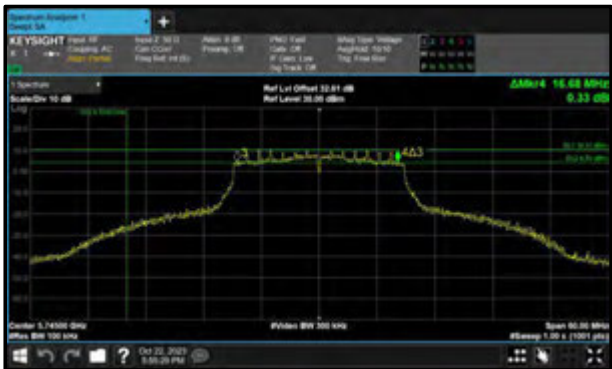
Figure 359 - 802.11ac VHT20 Minimum 6 dB EBW
