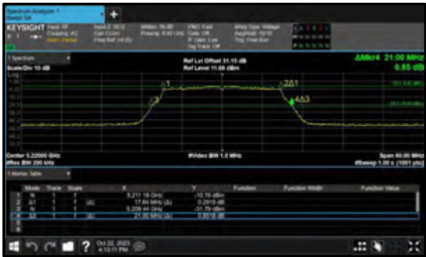
Figure 365 - 802.11ac VHT20 Minimum 99% OBW
