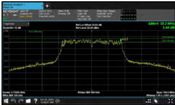
Figure 361 - 802.11ac VHT40 Minimum 6 dB EBW
