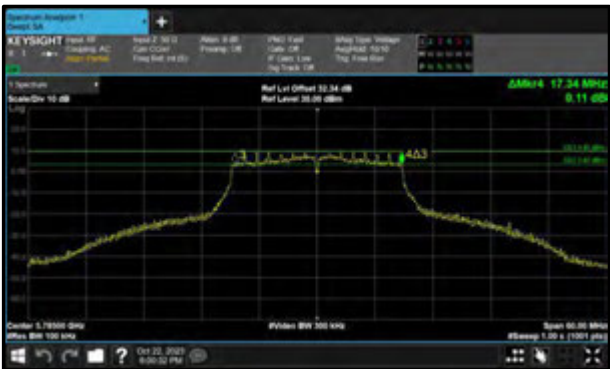
Figure 360 - 802.11ac VHT20 Maximum 6 dB EBW
