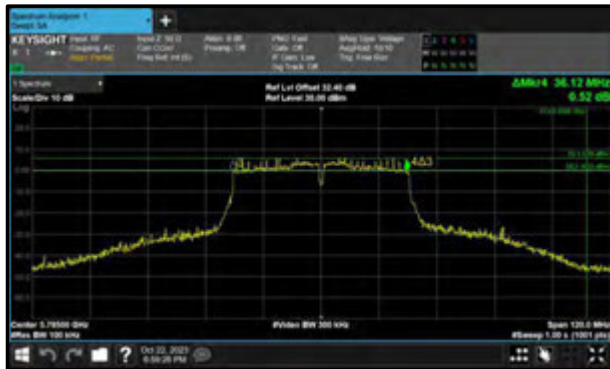
Figure 362 - 802.11ac VHT40 Maximum 6 dB EBW
