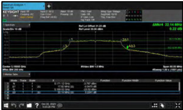
Figure 366 - 802.11ac VHT20 Maximum 99% OBW
