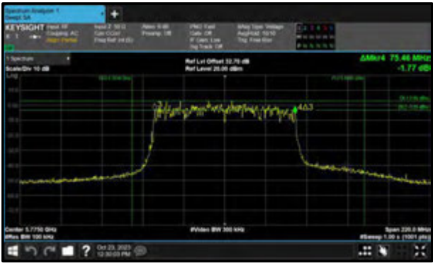
Figure 364 - 802.11ac VHT80 Maximum 6 dB EBW
