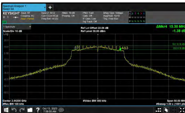
Figure 57 - 802.11n HT20 Minimum 6 dB EBW
