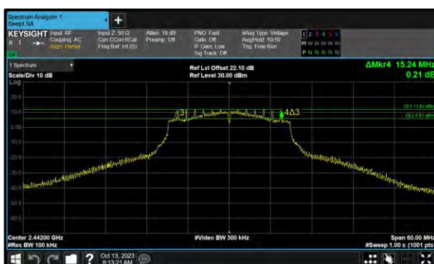
Figure 61 - 802.11n HT20 Minimum 6 dB EBW
