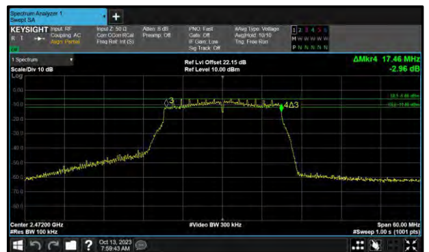
Figure 58 - 802.11n HT20 Maximum 6 dB EBW
