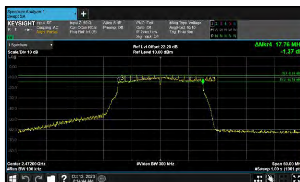
Figure 62 - 802.11n HT20 Maximum 6 dB EBW
