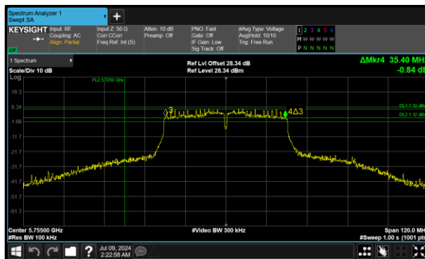
Figure 286 - 802.11n HT40 Minimum 6 dB EBW
