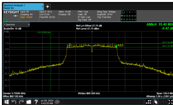
Figure 314 - 802.11n HT40 Minimum 6 dB EBW
