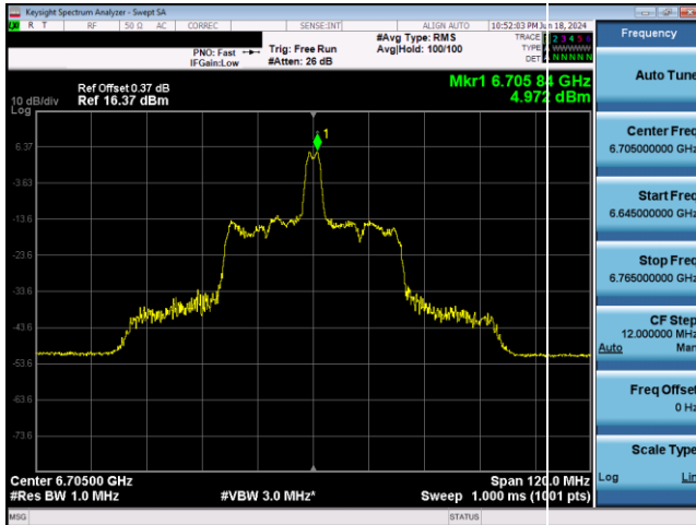
Plot 7-468. SP Power Spectral Density Plot Antenna 1b (80MHz 802.11ax RU26 (UNII Band 7) - Ch. 151)
