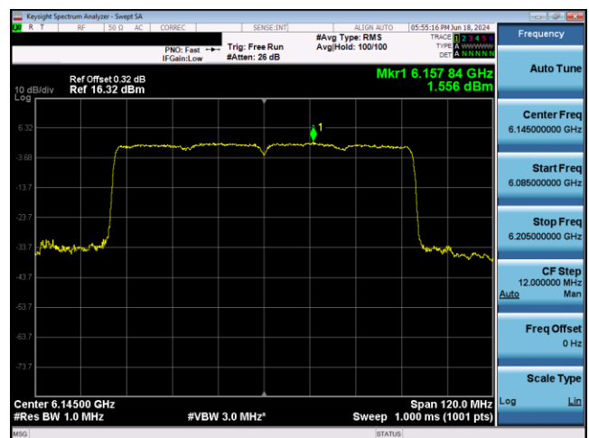
Plot 7-498. SP Power Spectral Density Plot CDD Antenna 3b (80MHz 802.11ax RU996 (UNII Band 5) – Ch. 39)
