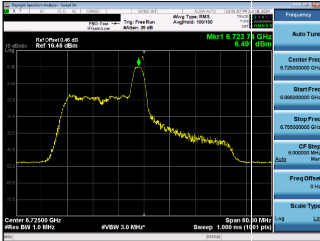
Plot 7-517. SP Power Spectral Density Plot CDD Antenna 5T (40MHz 802.11ax RU26 (UNII Band 7) – Ch. 155)
