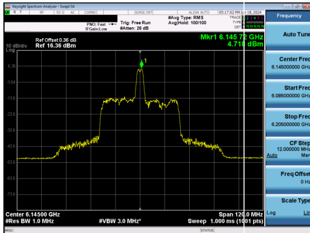
Plot 7-494. SP Power Spectral Density Plot CDD Antenna 3b (80MHz 802.11ax RU26 (UNII Band 5) – Ch. 39)
