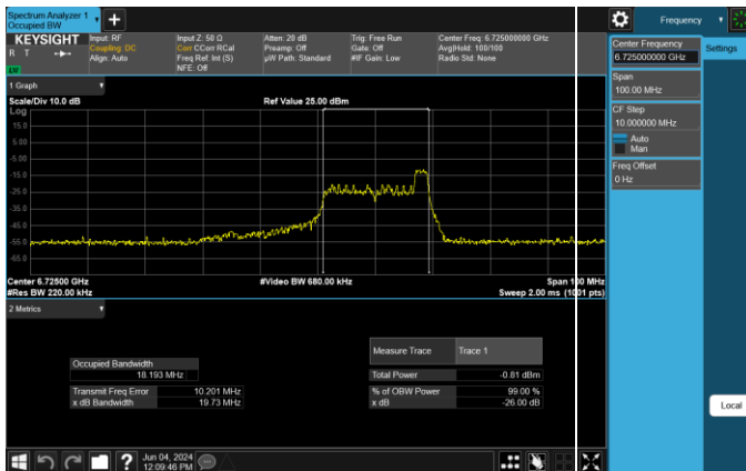
Plot 7-199. 26dB & 99% Bandwidth Plot Antenna 3b LPI (40MHz 802.11ax RU26 (UNII Band 7) – Ch. 155)
