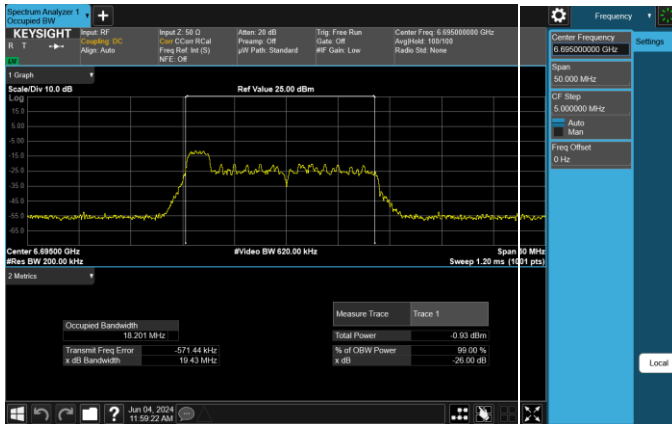
Plot 7-193. 26dB & 99% Bandwidth Plot Antenna 3b LPI (20MHz 802.11ax RU26 (UNII Band 7) – Ch. 149)
