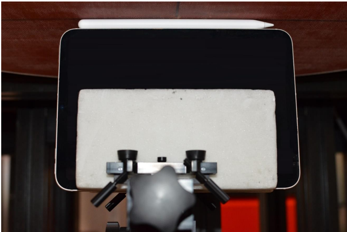
Wireless Power Transfer (wPT) Test Setup Photo 11: Body, Right Edge at 0.0mm
