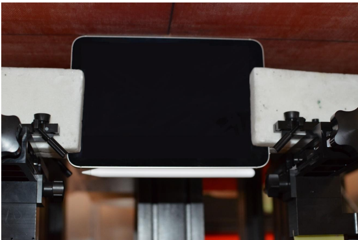
Wireless Power Transfer (wPT) Test Setup Photo 12: Body, Left Edge at 0.0mm
