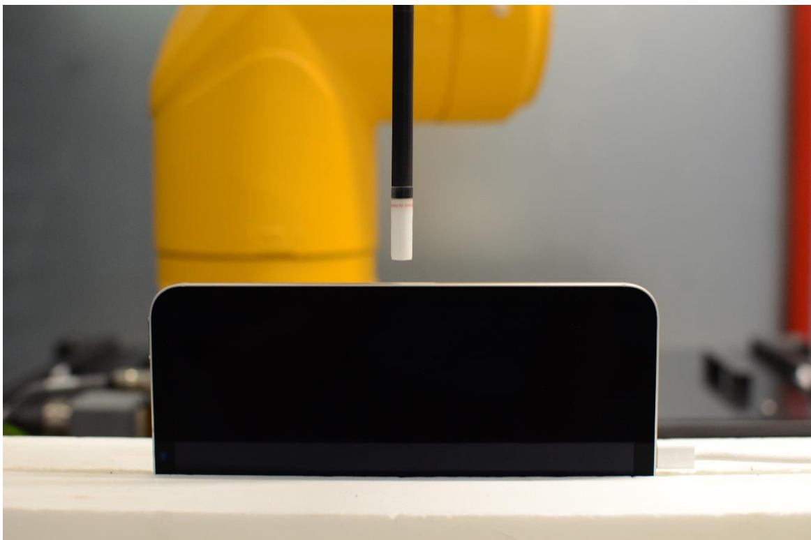
Near Field Power Density Test Setup 19: Body, Right Edge at 9.45mm – Ant 5T
