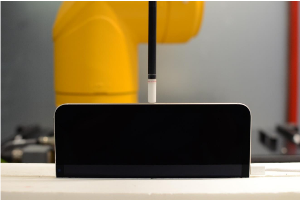
Near Field Power Density Test Setup 18: Body, Right Edge at 2mm – Ant 1b/3b/5T
