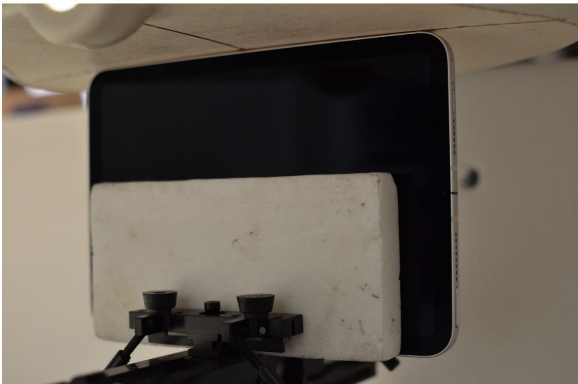
SAR Test Setup Photo 7: Body, Left Edge at 0.0 mm – Ant 1a/1b/2/3a/3b/5T
