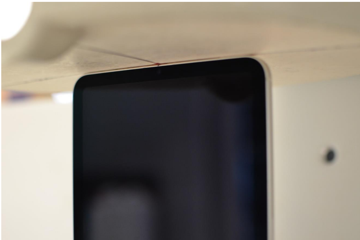
SAR Test Setup Photo 4: Body, Top Edge at 0.0 mm – Ant 3a/3b/4/5T
