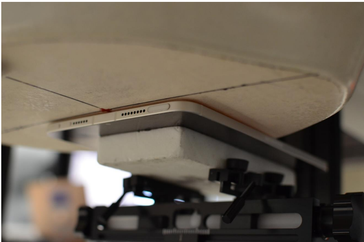
SAR Test Setup Photo 2: Body, Back Side at 0.0 mm – Ant 3a/3b/4
