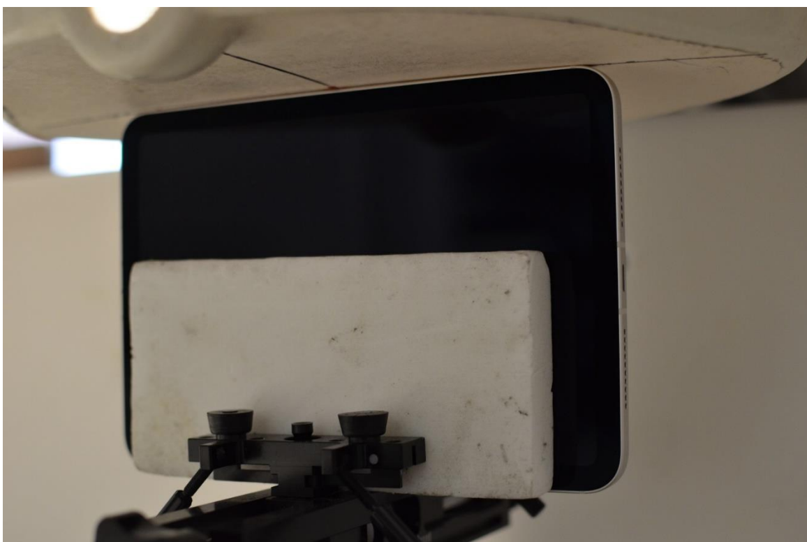
SAR Test Setup Photo 6: Body, Right Edge at 0.0 mm – Ant 1a/1b/2/3a/3b/5T
