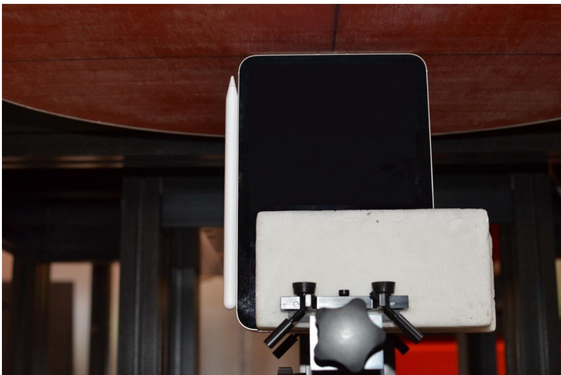
Wireless Power Transfer (wPT) Test Setup Photo 10: Body, Bottom Edge at 0.0mm
