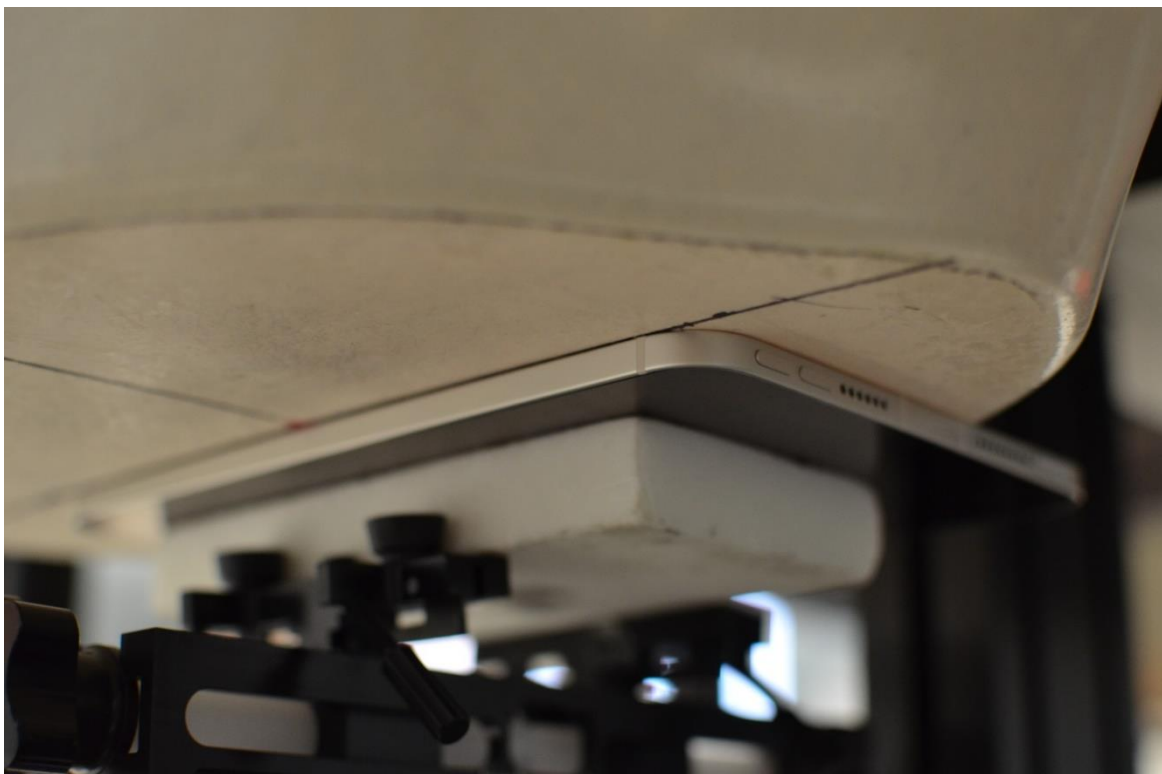
SAR Test Setup Photo 1: Body, Back Side at 0.0 mm – Ant 5T
