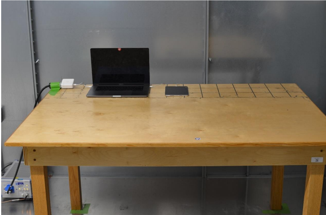
Figure 3: AC Line Conducted Emissions (Front View)
