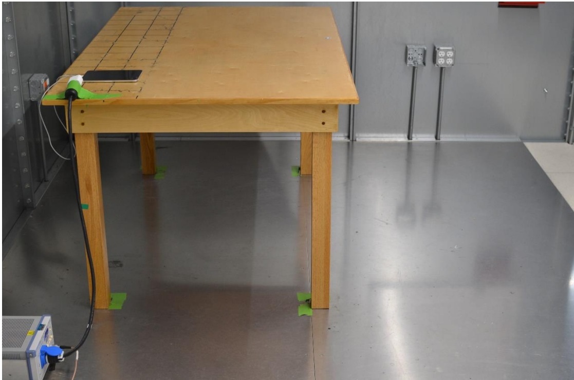
Figure 2: AC Line Conducted Emissions (Side View)
