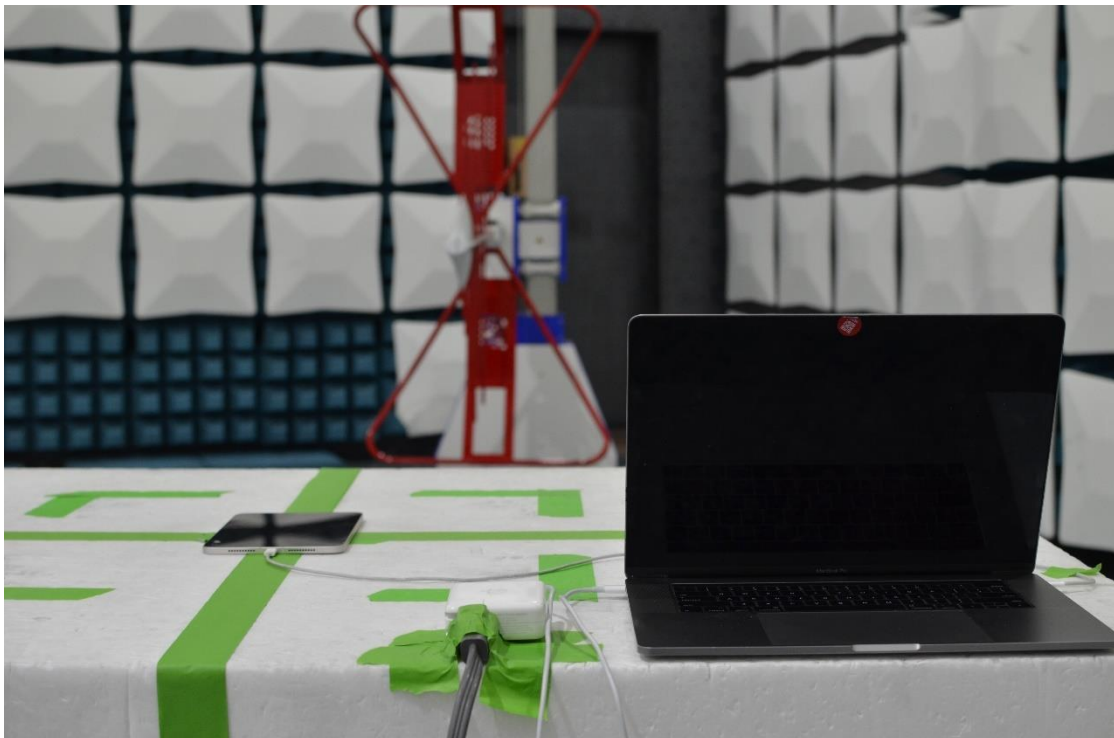
Figure 18: 30MHz-1GHz Test Setup (Rear View)
