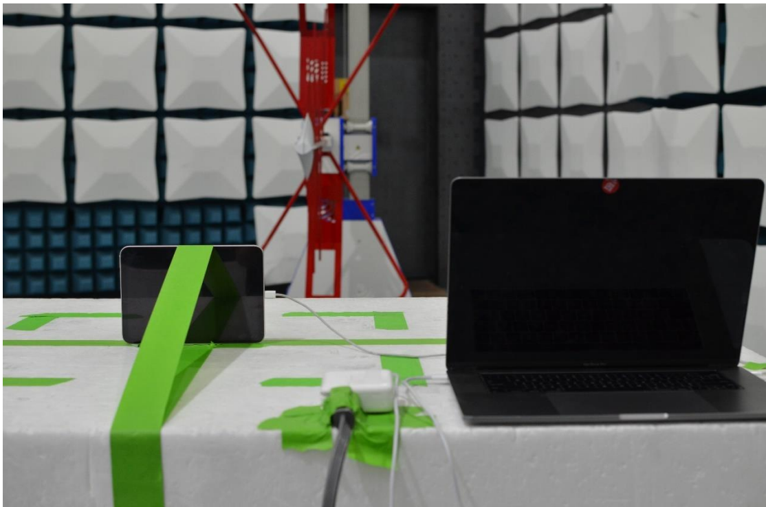
Figure 20: 30MHz-1GHz Test Setup (Rear View)
