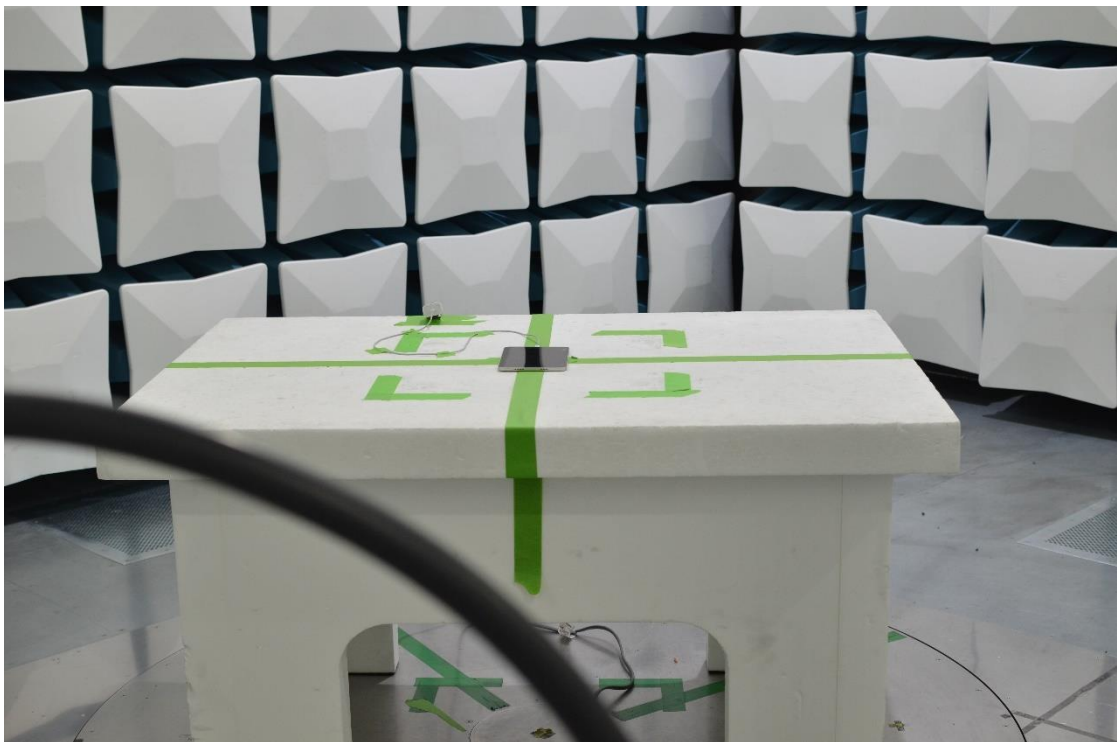
Figure 23: 9kHz-30MHz Test Setup (Front View)
