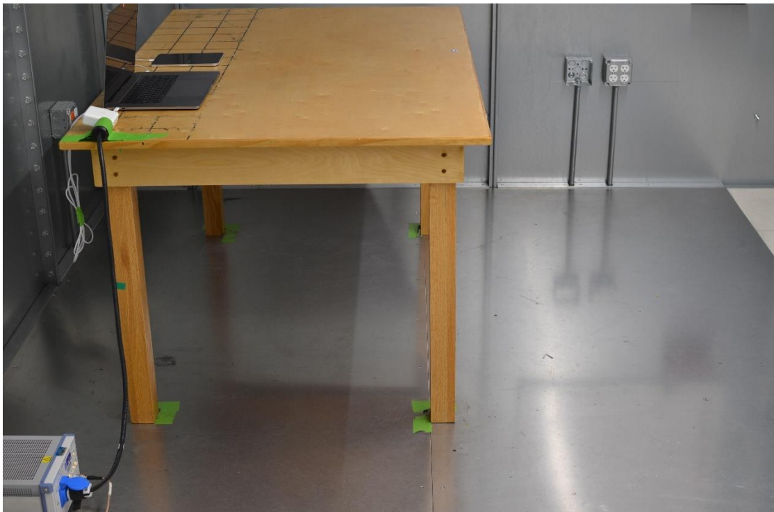
Figure 4: AC Line Conducted Emissions (Side View)
