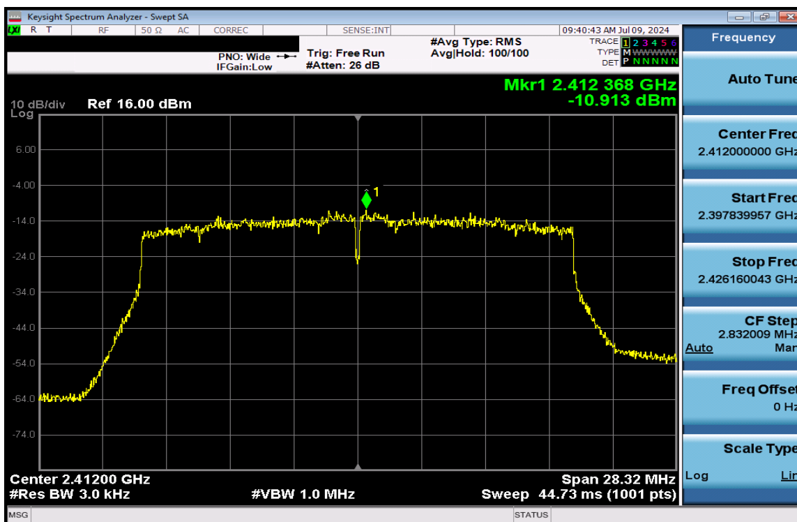
Plot 7-106. Power Spectral Density Plot Antenna 1a (802.11ax (SU - 2.4GHz) – Ch. 1) – MCS4
