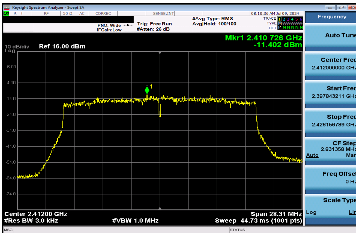
Plot 7-151. Power Spectral Density Plot CDD Antenna 3a (802.11ax (SU - 2.4GHz) – Ch. 1) – MCS4
