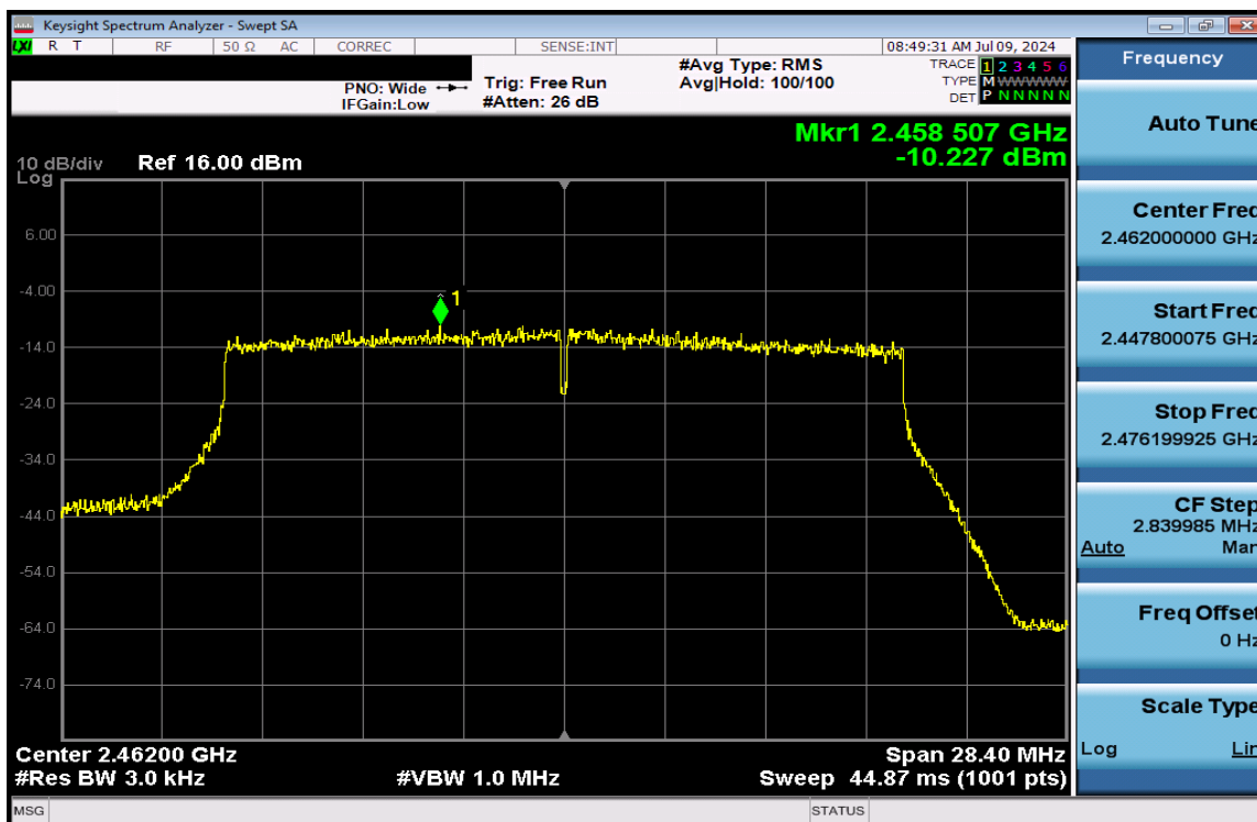
Plot 7-138. Power Spectral Density Plot CDD Antenna 1a (802.11ax (SU - 2.4GHz) – Ch. 11) – MCS2
