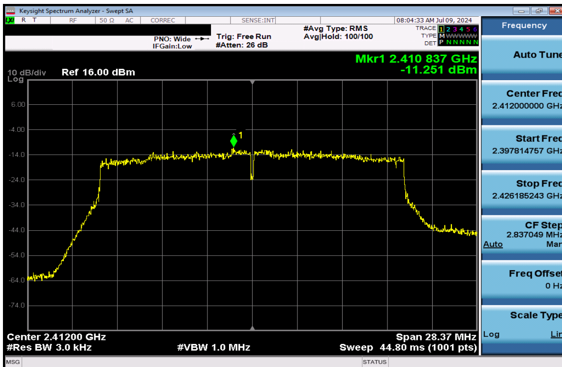
Plot 7-133. Power Spectral Density Plot CDD Antenna 3a (802.11ax (SU - 2.4GHz) – Ch. 1) – MCS2
