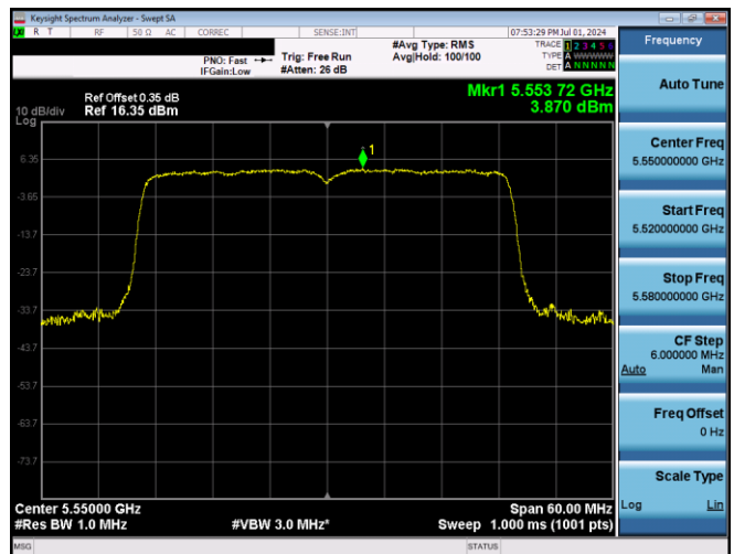
Plot 7-422. PSD Antenna 3b (40MHz BW 802.11ax(SU) – Ch. 110, MCS11)
