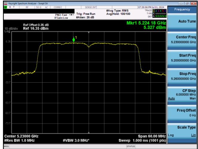
Plot 7-408. PSD Antenna 3b (40MHz BW 802.11ax(SU) – Ch. 46, MCS11)
