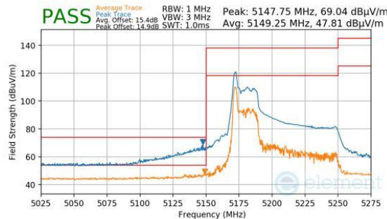
Plot 7-838. Antenna 5T (Peak & Average, RU26, Index 0, Ch.42, MCS11)
