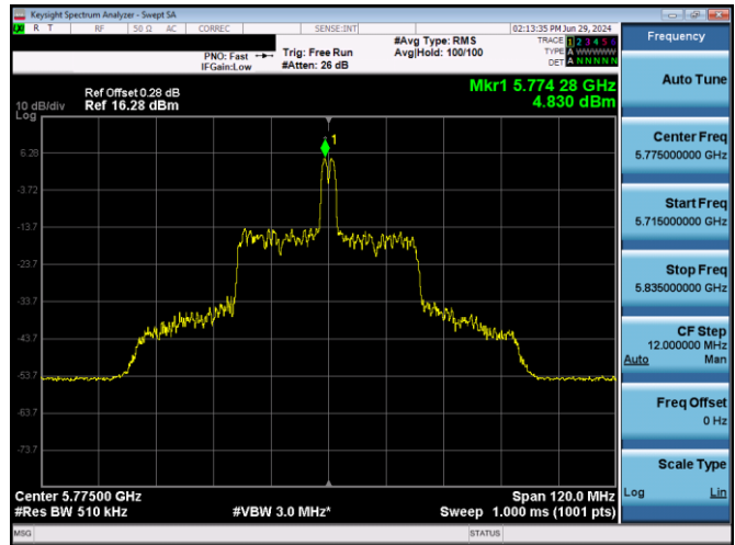
Plot 7-293. PSD Antenna 3b (80MHz BW 11ax Index 18 - RU26 - Ch.155)
