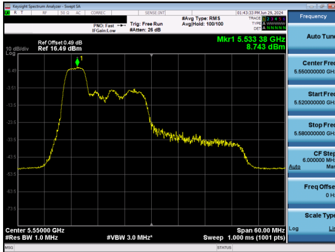
Plot 7-272. PSD Antenna 3b (40MHz BW 11ax Index 37 - RU52 - Ch.110)
