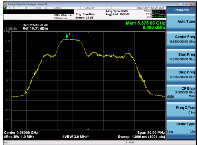
Plot 7-269. PSD Antenna 3b (20MHz BW 11ax Index 38 – RU52 – Ch.116)
