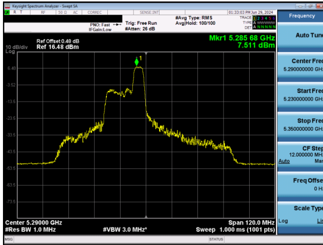
Plot 7-265. PSD Antenna 3b (80MHz BW 11ax Index 44 – RU52 – Ch.58)
