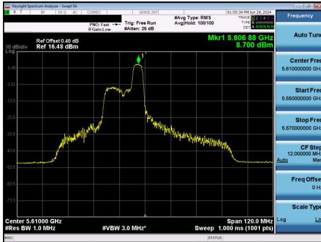
Plot 7-277. PSD Antenna 3b (80MHz BW 11ax Index 44 - RU52 - Ch.122)
