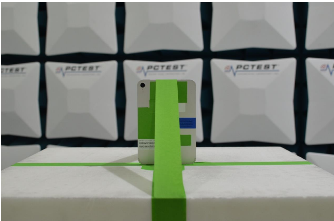
Figure 5: 1-18GHz Test Setup (Front View)
