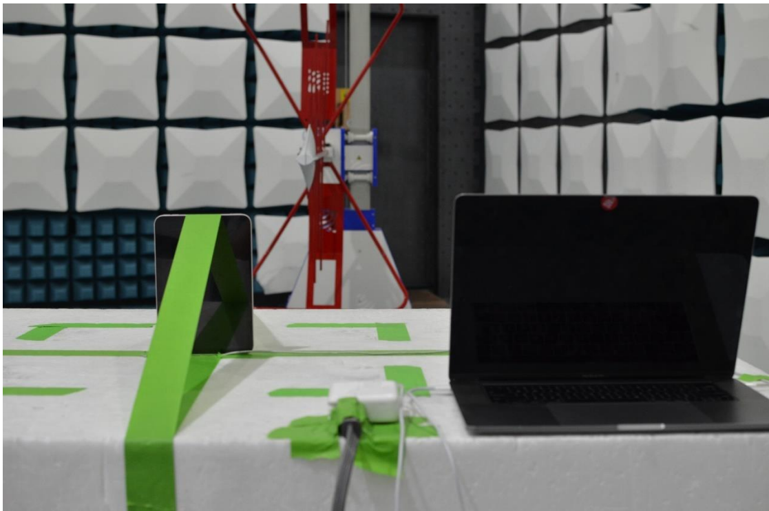
Figure 18: 30MHz-1GHz Test Setup (Rear View)
