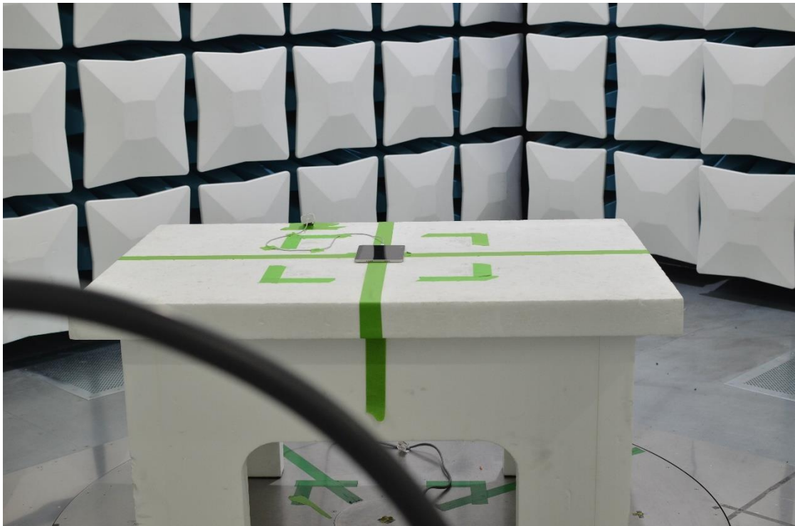
Figure 19: 9kHz-30MHz Test Setup (Front View)
