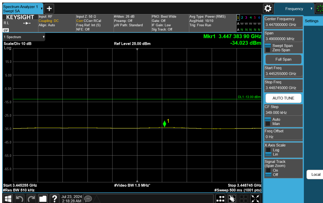
Plot 7-186. Lower ACP Plot (NR Band n77 DoD-Band - 70MHz DFT-s-OFDM QPSK – Full RB)
