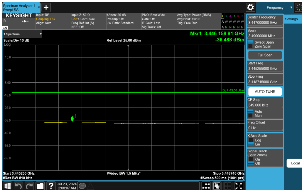
Plot 7-178. Lower ACP Plot (NR Band n77 DoD-Band - 60MHz DFT-s-OFDM QPSK – Full RB)
