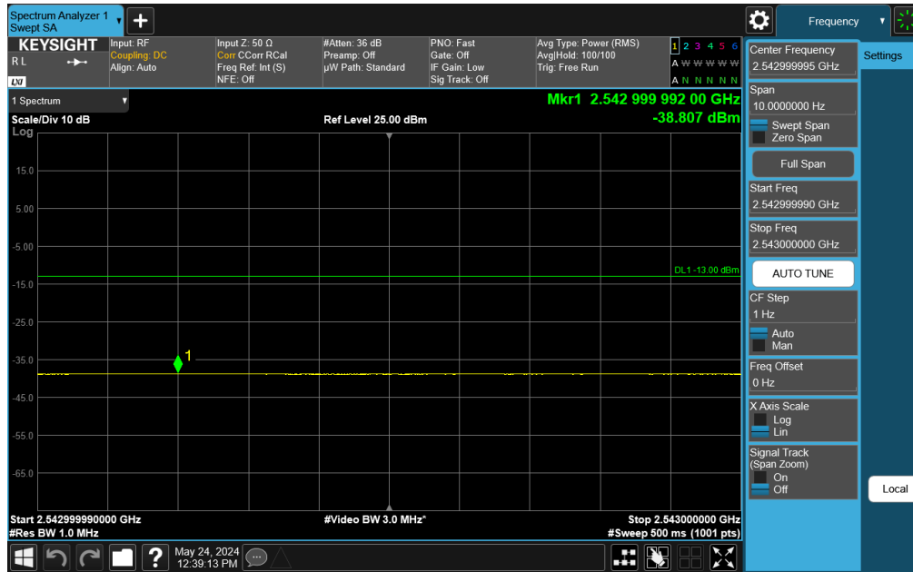
Plot 7-393. Middle Band Edge Plot (NR Band n7 - 5MHz DFT-s-OFDM QPSK – Full RB)
