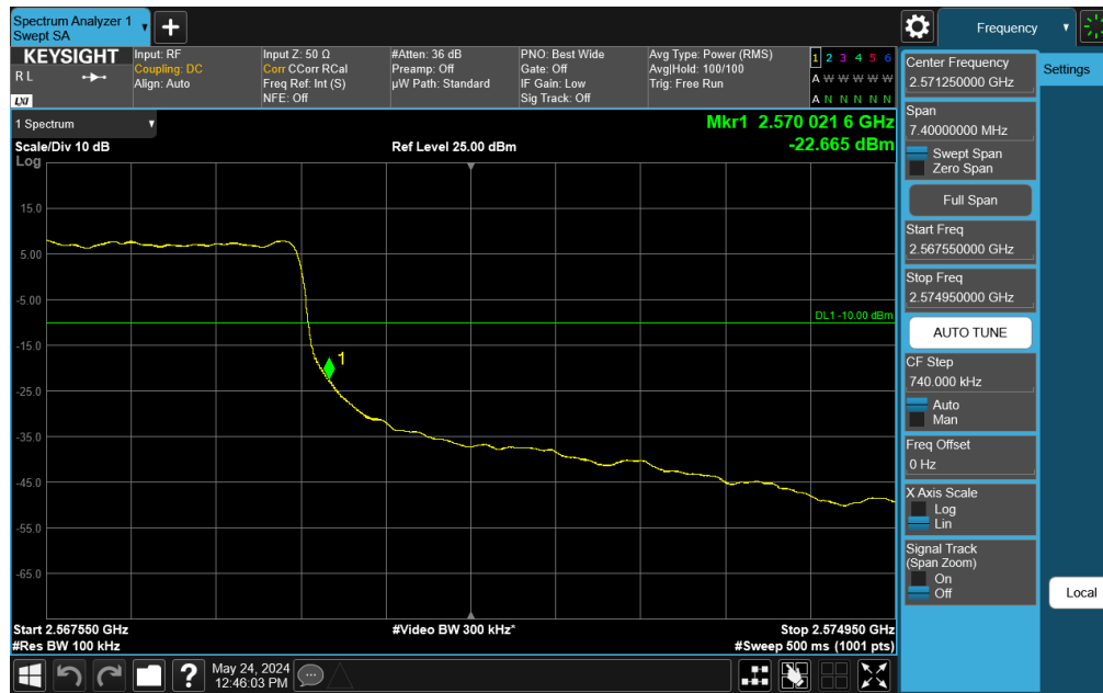
Plot 7-399. Upper Band Edge Plot (NR Band n7 - 5MHz DFT-s-OFDM QPSK – Full RB)
