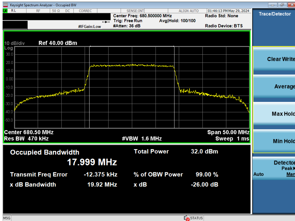
Plot 7-39. Occupied Bandwidth Plot (LTE Band 71 - 20MHz 64-QAM - Full RB)
