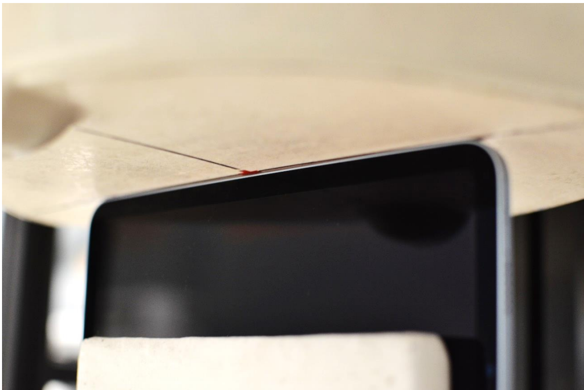
SAR Test Setup Photo 7: Left Edge at 0mm – Ant WF8/WF7/WF5T/WF2
