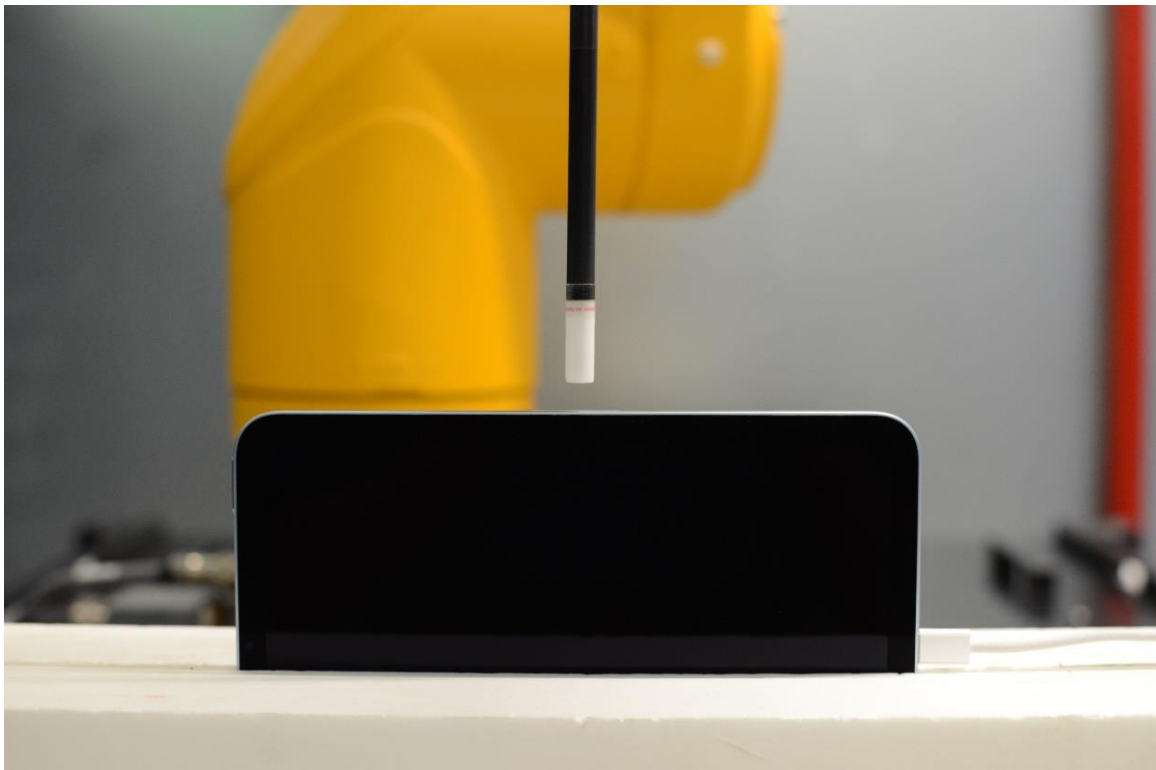
Near Field Power Density Test Setup Photo 19: Right Edge at 9.45mm – WF5T
