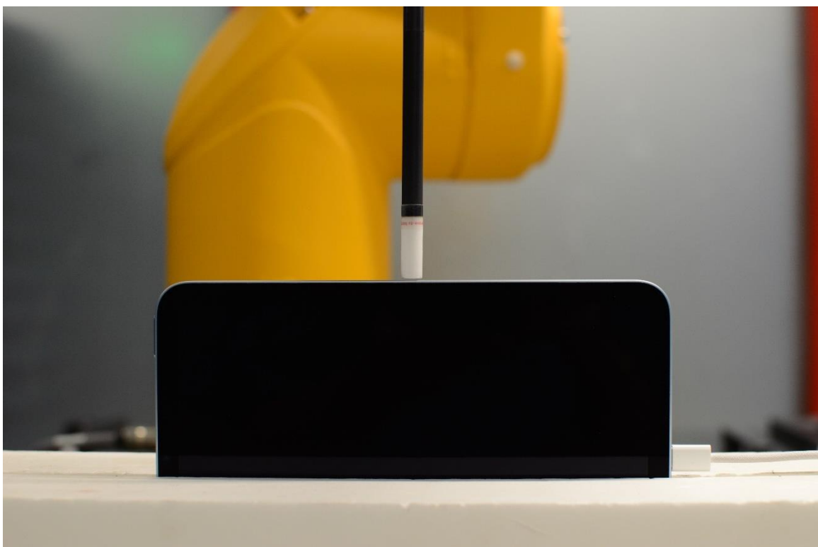
Near Field Power Density Test Setup Photo 18: Right Edge at 2mm – WF5T/WF2
