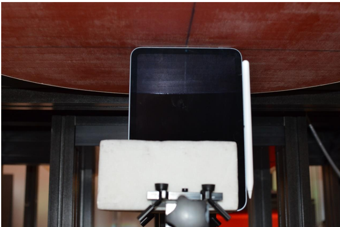
Wireless Power Transfer (wPT) Test Setup Photo 9: Top Edge at 0mm
