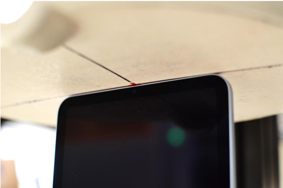
SAR Test Setup Photo 4: Top Edge at 0mm – Ant WF8/WF7/WF5T/WF2
