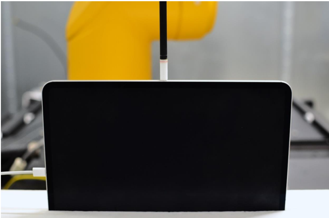
Near Field Power Density Test Setup 14: Left Edge at 2mm – Antenna 2a/4a/WF5B
