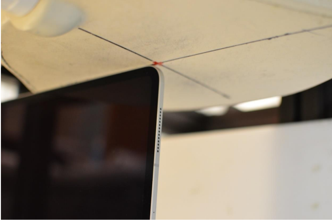
SAR Test Setup Photo 7: Body, Left Edge at 0mm – Antenna 3/4a/4b
