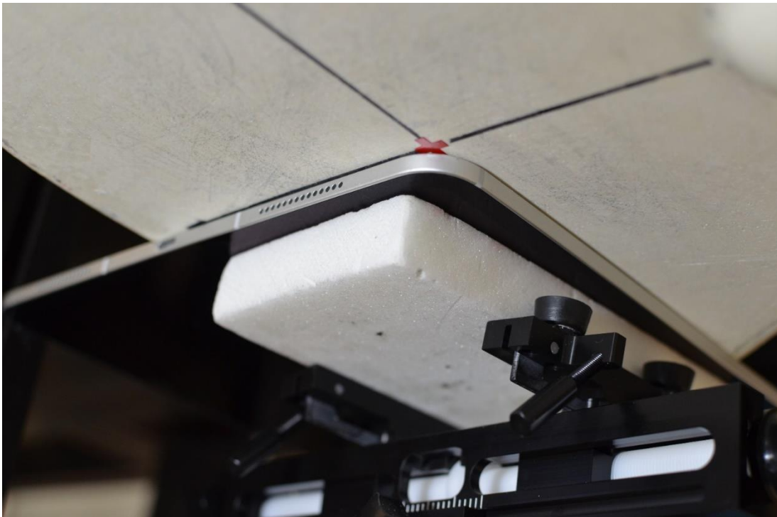
SAR Test Setup Photo 2: Body, Back Side at 0mm– Antenna 1/2a/2b/WF5B
