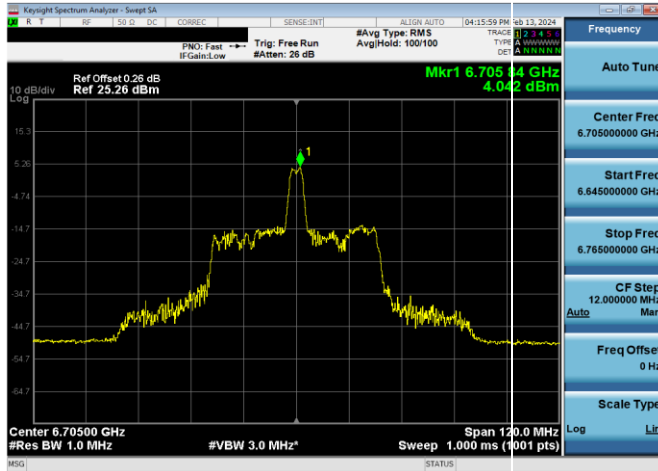
Plot 7-282. SP Power Spectral Density Plot Antenna 2a (80MHz 802.11ax RU26 (UNII Band 7) - Ch. 151)
