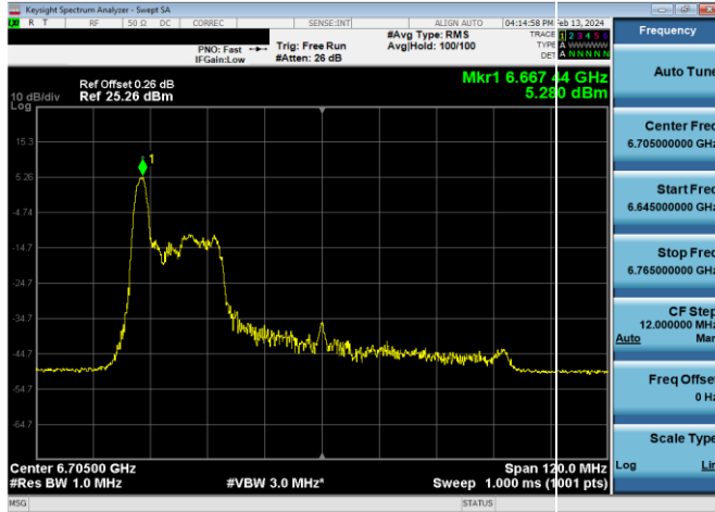
Plot 7-281. SP Power Spectral Density Plot Antenna 2a (80MHz 802.11ax RU26 (UNII Band 7) - Ch. 151)
