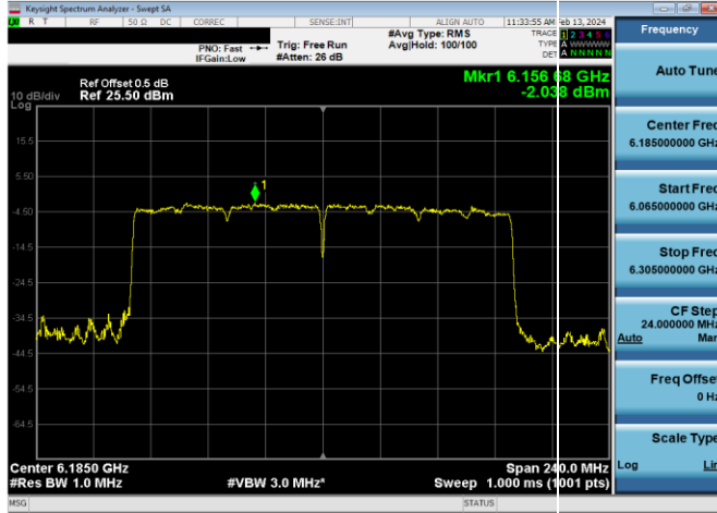
Plot 7-320. SP Power Spectral Density Plot CDD Primary Antenna 4a (160MHz 802.11ax RU996x2 (UNII Band 5) – Ch. 47)
