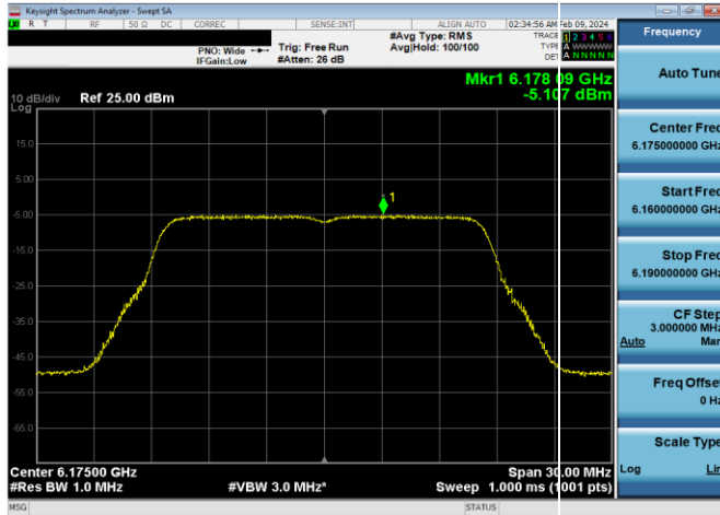
Plot 7-361. Power Spectral Density Plot Antenna 2a LPI (20MHz 802.11a (UNII Band 5) – Ch. 45, 12Mbps)
