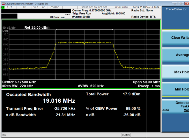
Plot 7-82. 26dB & 99% Bandwidth Plot Antenna 4a (20MHz 802.11ax (UNII Band 5) – Ch. 45, MCS4)
