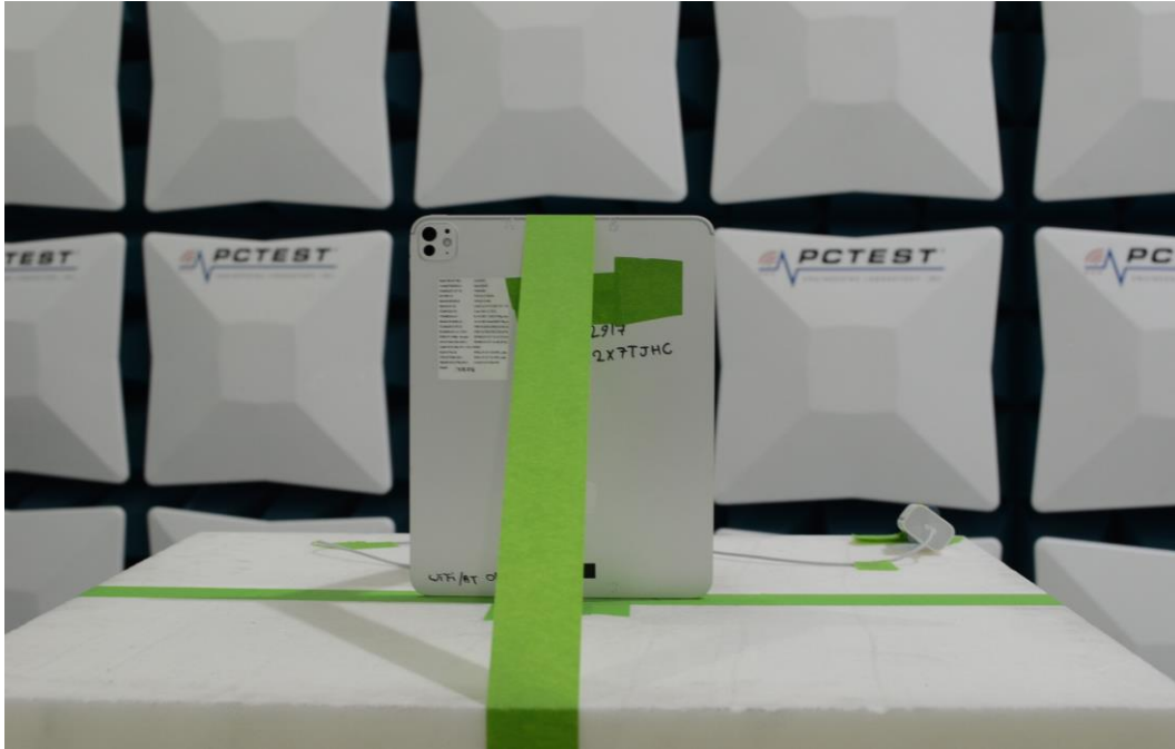
Figure 9: 1-18GHz Test Setup (Front View)
