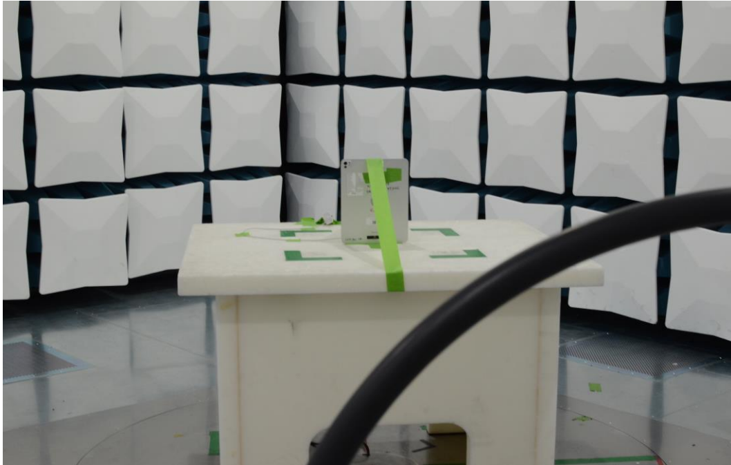
Figure 25: 9kHz-30MHz Test Setup (Front View)
