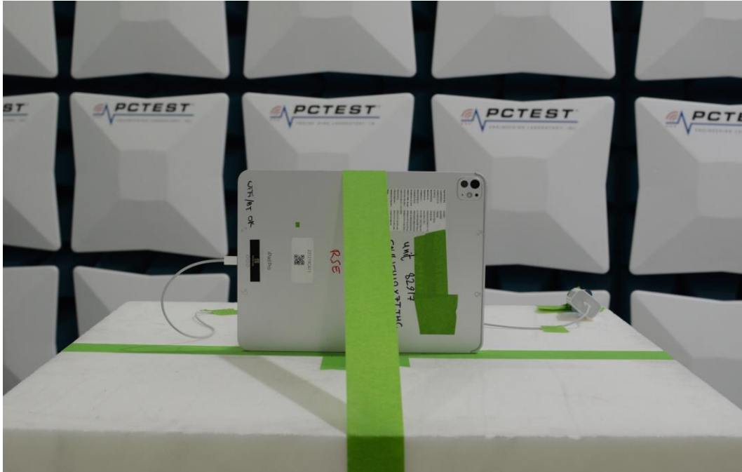
Figure 7: 1-18GHz Test Setup (Front View)
