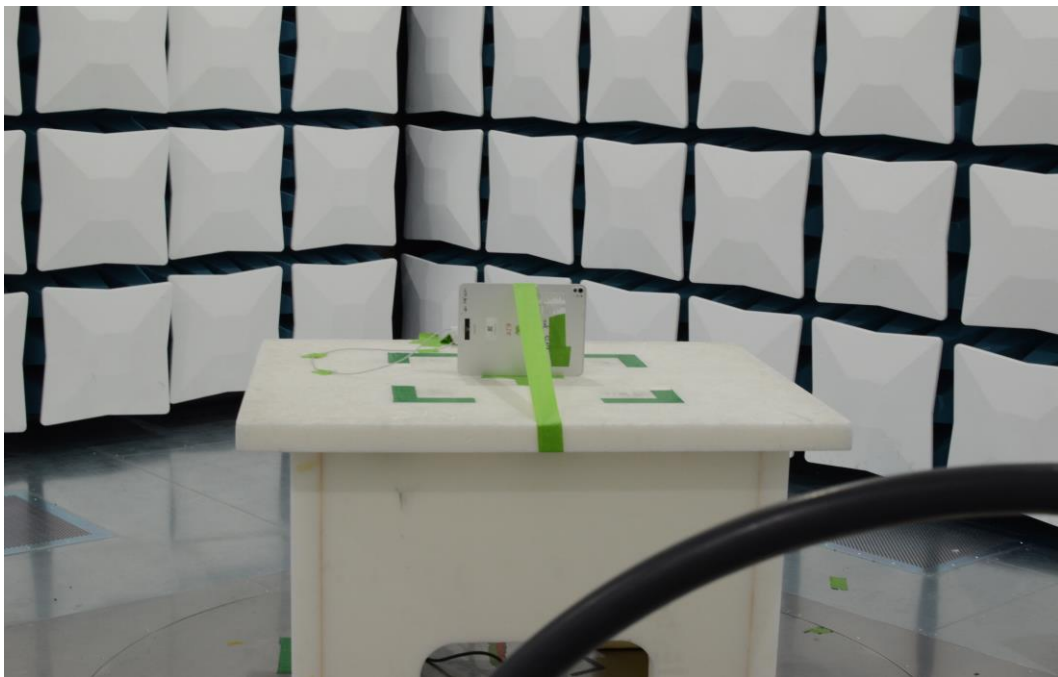
Figure 24: 9kHz-30MHz Test Setup (Front View)
