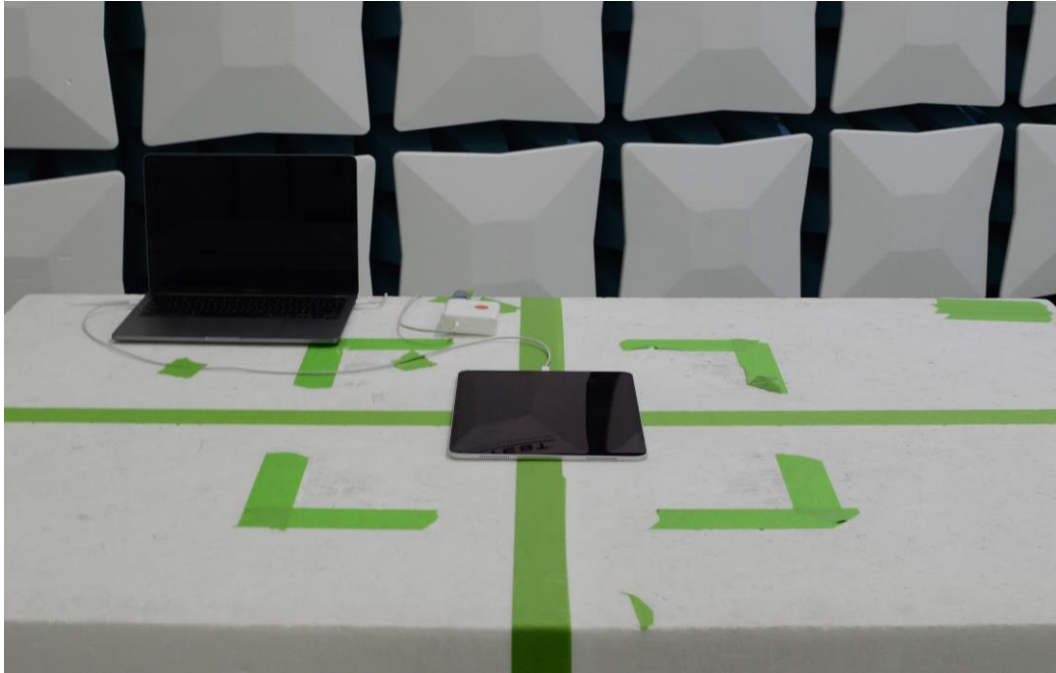
Figure 17: 30MHz-1GHz Test Setup (Front View)
