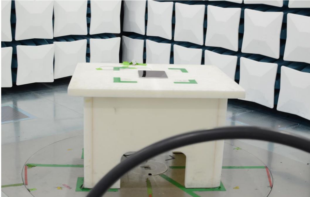
Figure 23: 9kHz-30MHz Test Setup (Front View)
