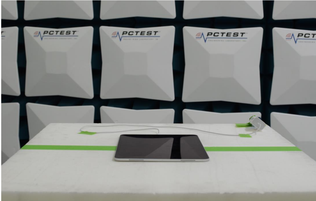
Figure 5: 1-18GHz Test Setup (Front View)
