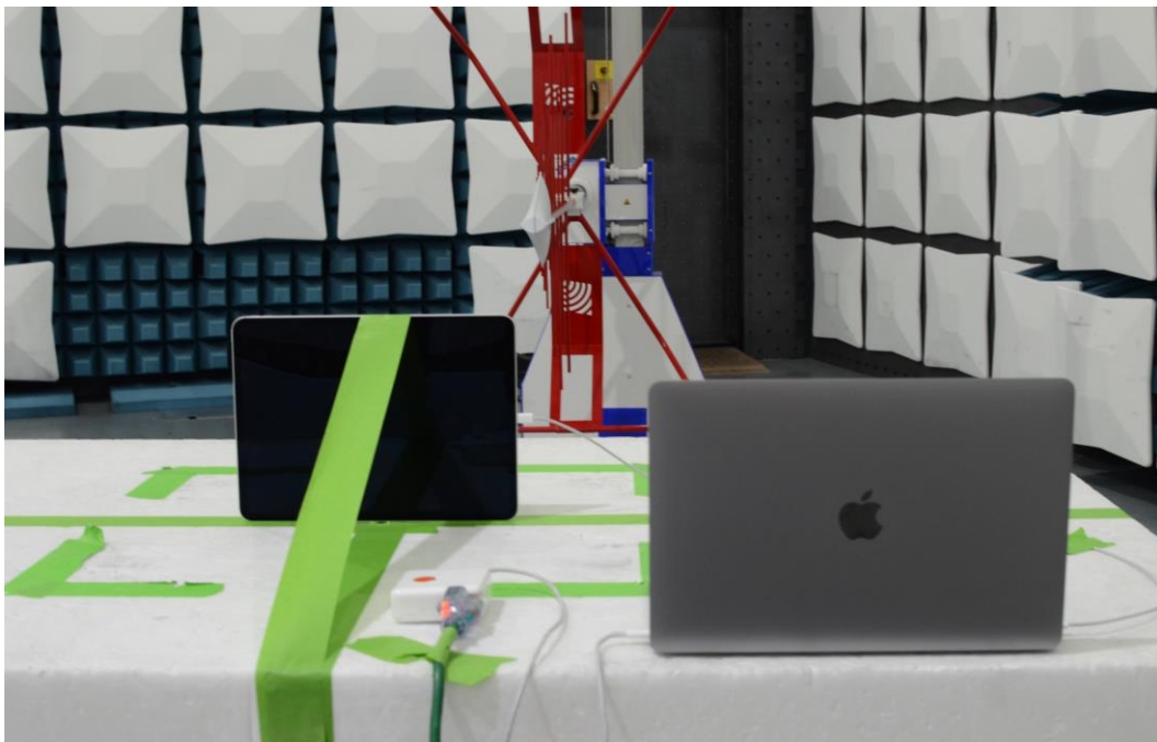
Figure 20: 30MHz-1GHz Test Setup (Rear View)
