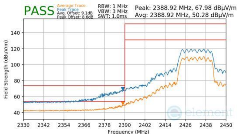
Plot 7-866 Radiated Restricted Lower Band Edge Measurement CDD Primary
