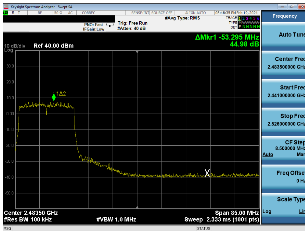
Plot 7-456. Band Edge Plot Antenna WF7 (802.11ax (SU - 2.4GHz) – Ch. 9) – MCS9
