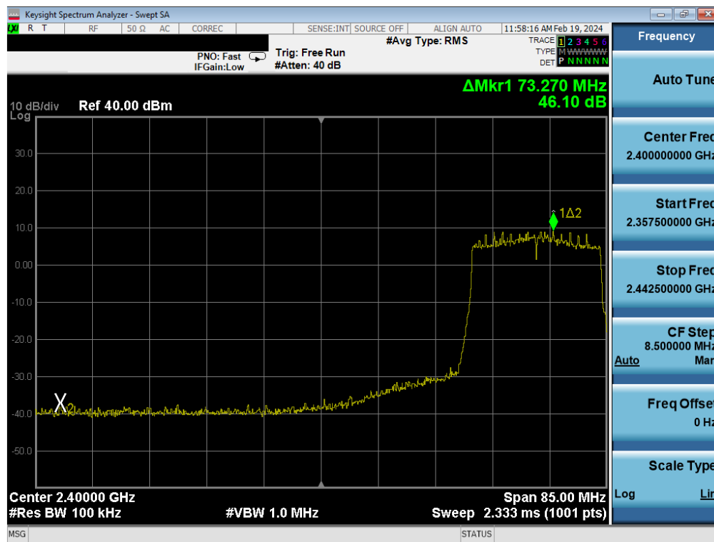
Plot 7-282. Band Edge Plot Antenna WF8 (802.11ax (SU - 2.4GHz) – Ch. 5) – MCS2
