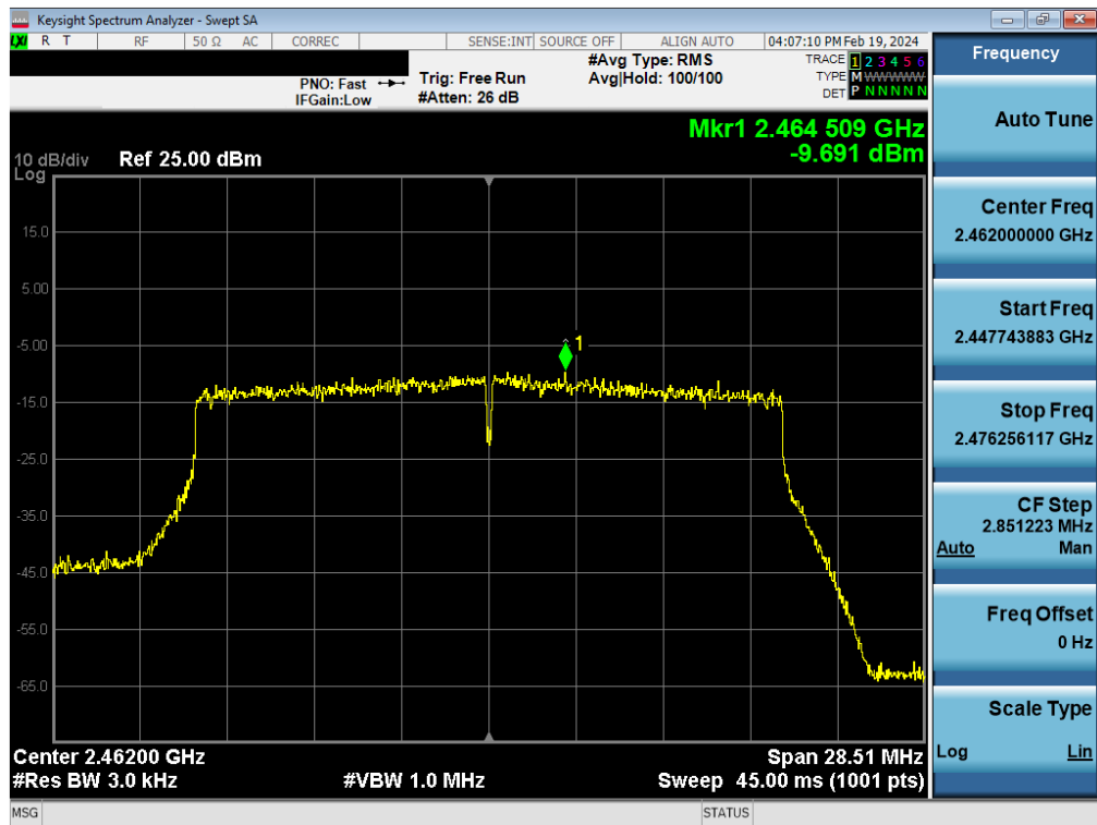
Plot 7-129. Power Spectral Density Plot Antenna WF7 (802.11ax (SU - 2.4GHz) – Ch. 11) – MCS2
