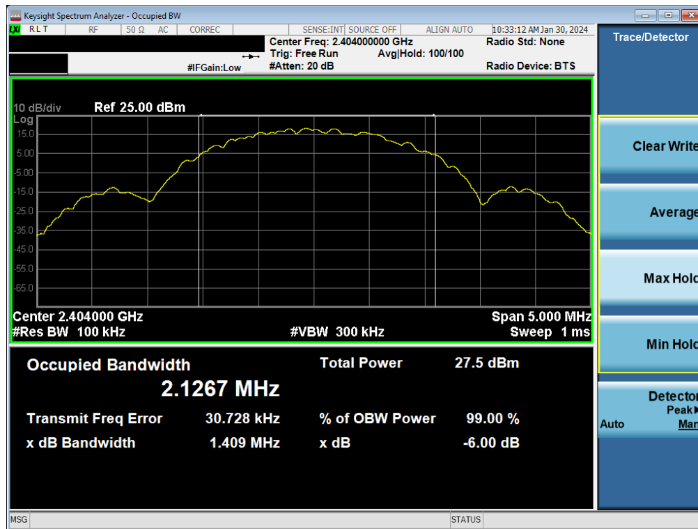
Plot 7-16. 6dB BW & 99% OBW Plot Antenna WF9 (Bluetooth (LE), 2Mbps, ePA – Ch. 1)
