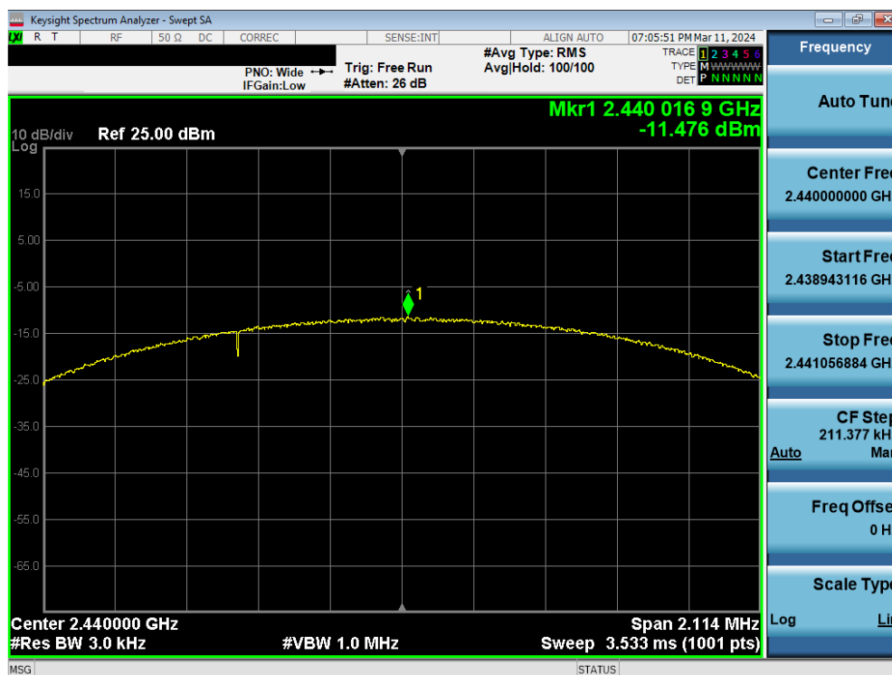
Plot 7-29. Power Spectral Density Plot Antenna WF8 (Bluetooth (LE), 2Mbps, iPA – Ch. 19)
