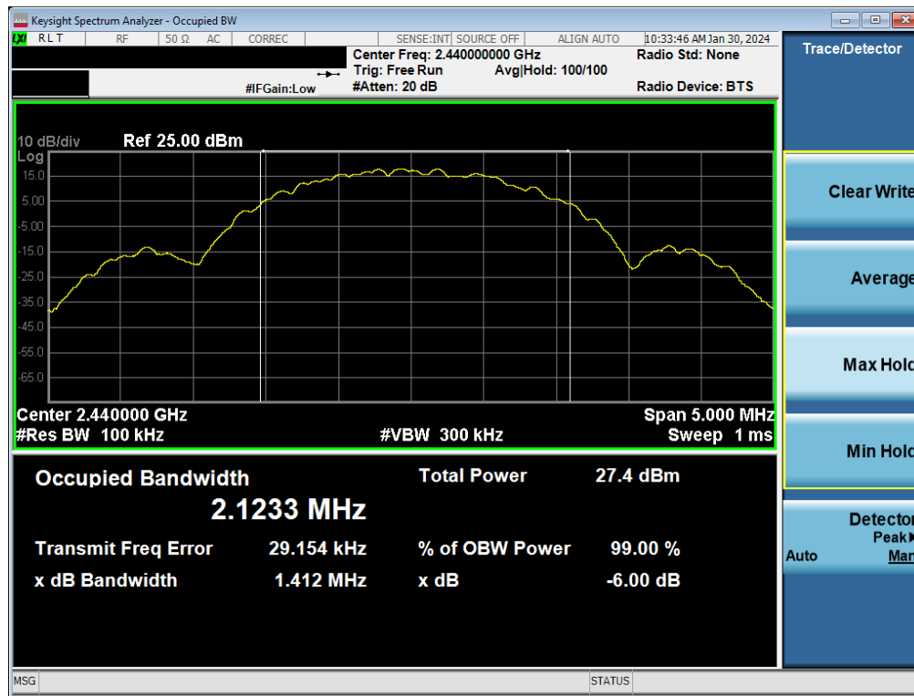
Plot 7-17. 6dB BW & 99% OBW Plot Antenna WF9 (Bluetooth (LE), 2Mbps, ePA – Ch. 19)
