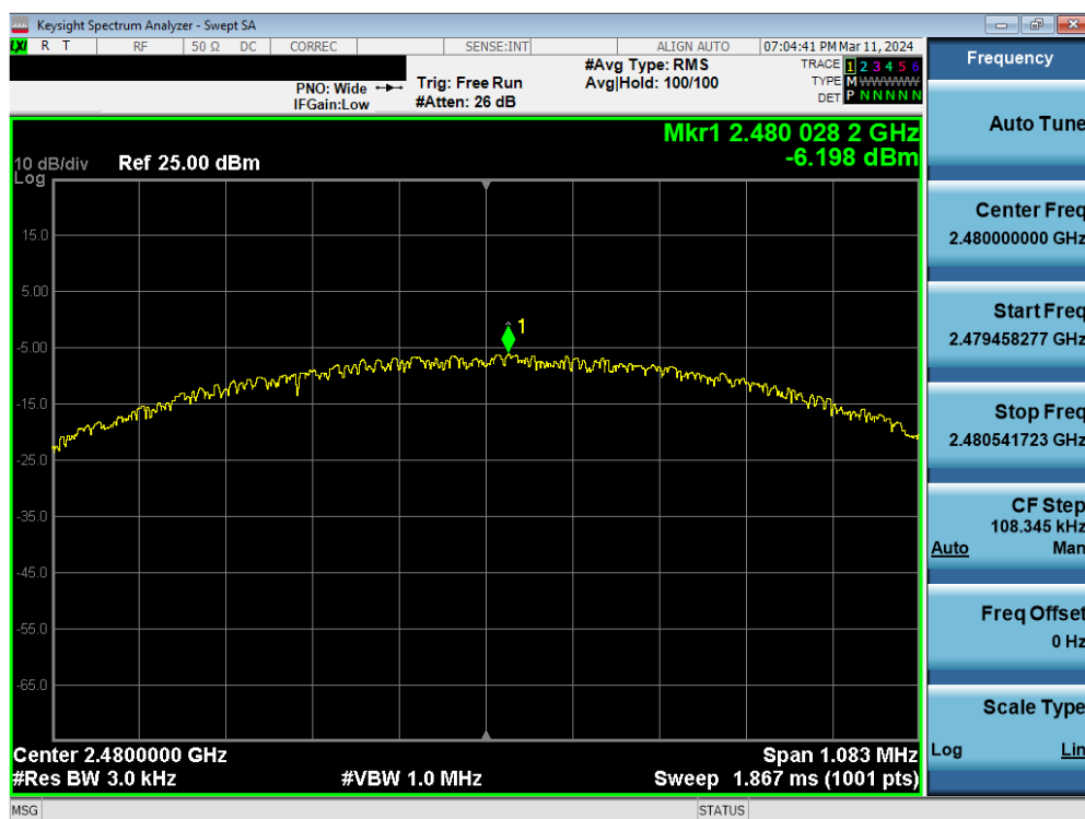
Plot 7-24. Power Spectral Density Plot Antenna WF8 (Bluetooth (LE), 1Mbps, iPA – Ch. 39)
