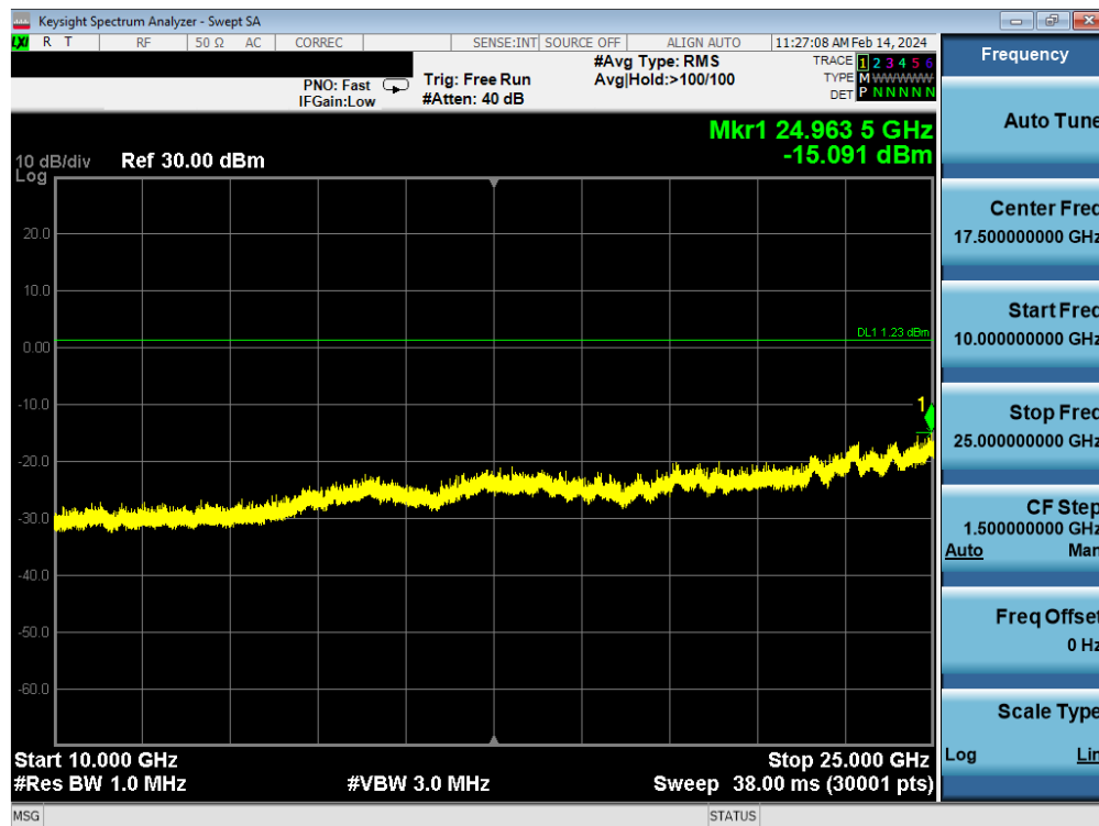
Plot 7-94. Conducted Spurious Plot Antenna WF8 (Bluetooth (LE), 1Mbps, ePA – Ch. 19)
