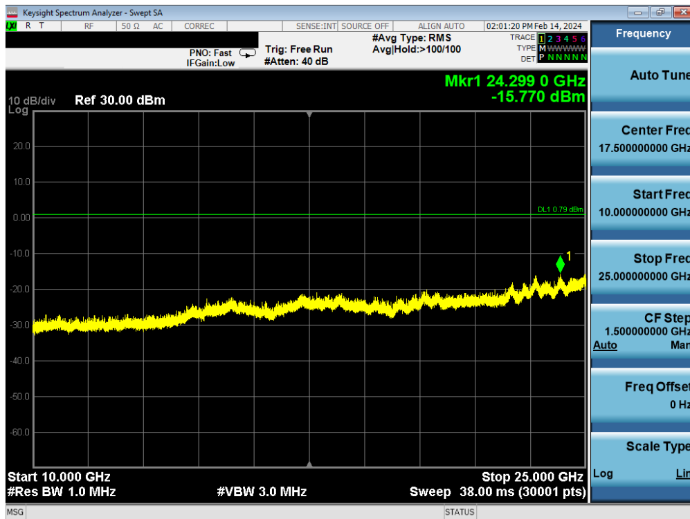
Plot 7-102. Conducted Spurious Plot Antenna WF7 (Bluetooth (LE), 1Mbps, ePA – Ch. 39)
