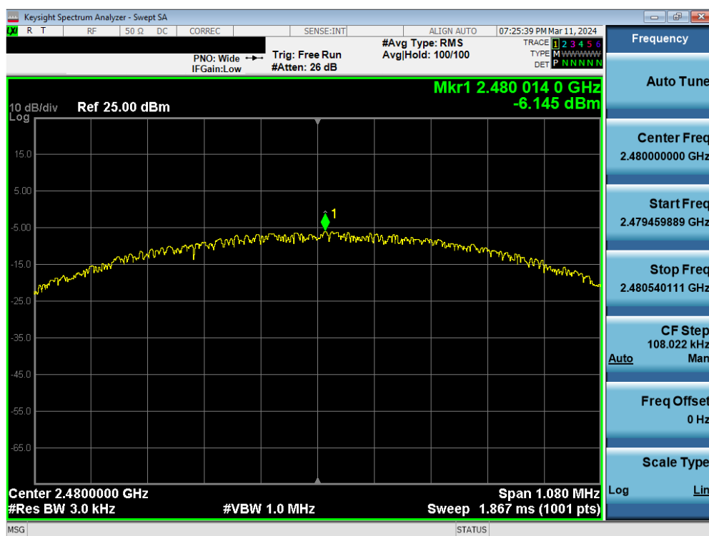
Plot 7-33. Power Spectral Density Plot Antenna WF7 (Bluetooth (LE), 1Mbps, ePA – Ch. 39)
