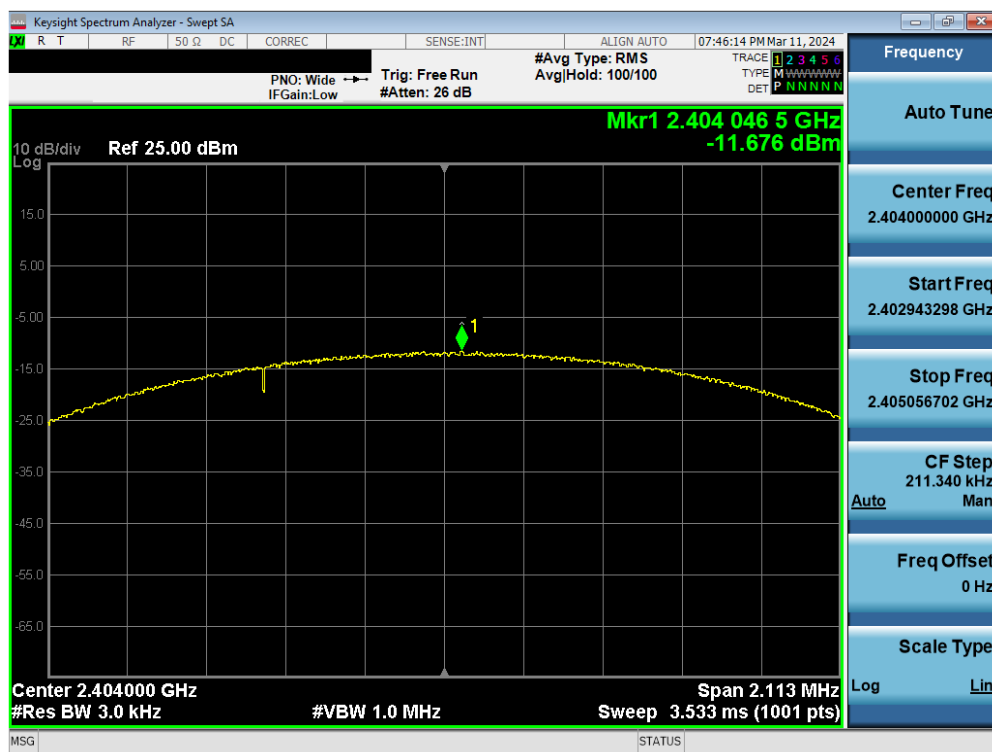
Plot 7-52. Power Spectral Density Plot Antenna WF9 (Bluetooth (LE), 2Mbps, iPA – Ch. 1)
