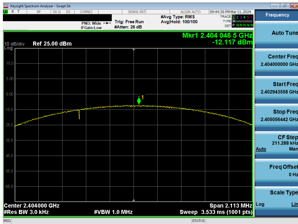
Plot 7-73. Power Spectral Density Plot Antenna WF8 (Bluetooth (LE), 2Mbps, iPA – Ch. 1)
