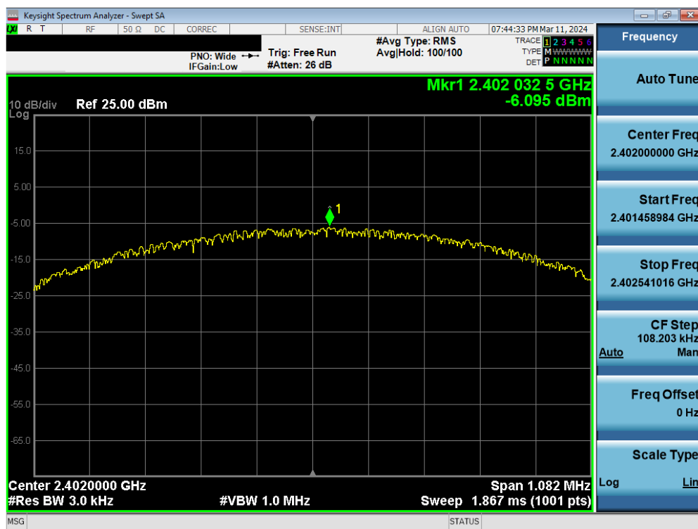
Plot 7-46. Power Spectral Density Plot Antenna WF9 (Bluetooth (LE), 1Mbps, iPA – Ch. 0)
