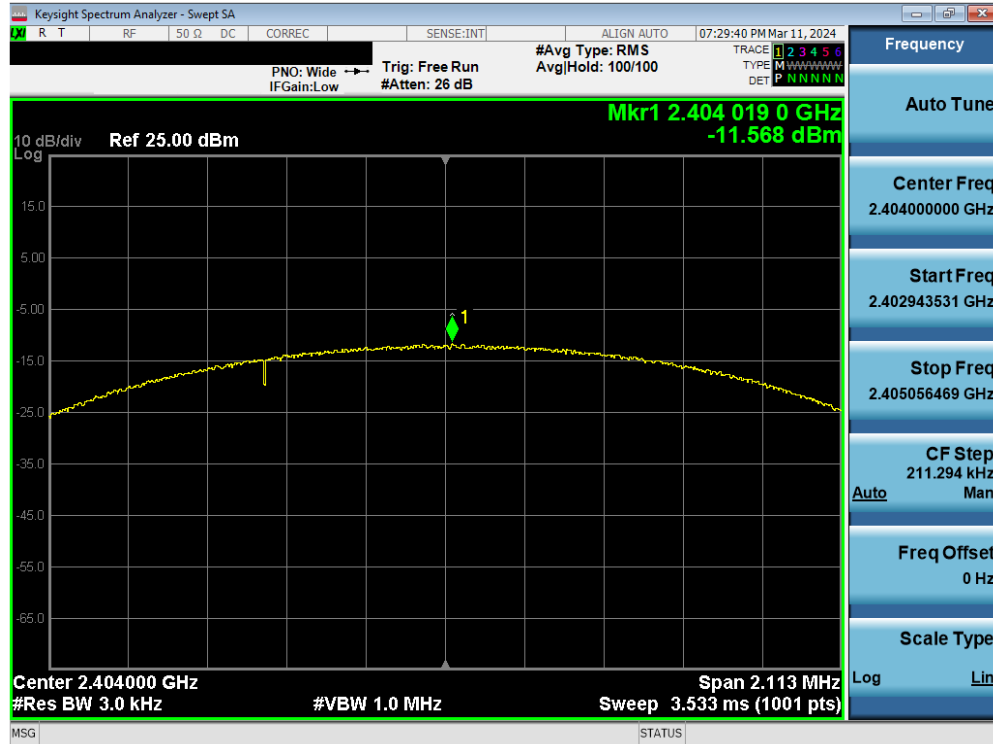
Plot 7-40. Power Spectral Density Plot Antenna WF7 (Bluetooth (LE), 2Mbps, iPA – Ch. 1)
