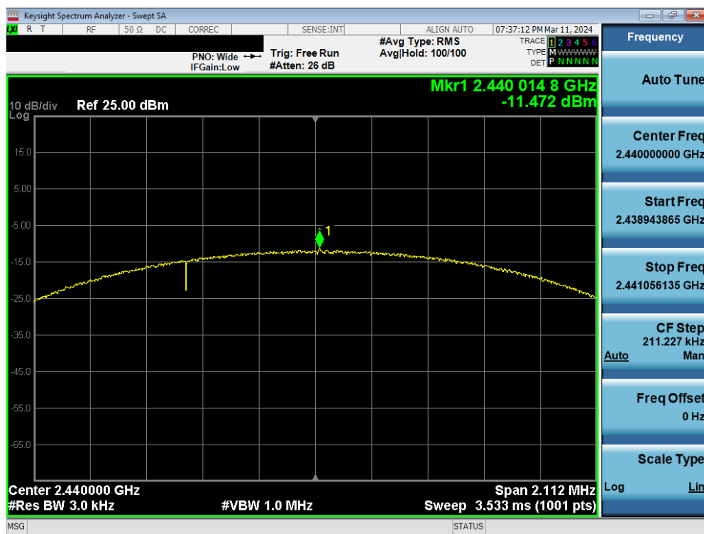
Plot 7-76. Power Spectral Density Plot Antenna WF7 (Bluetooth (LE), 2Mbps, iPA – Ch. 19)
