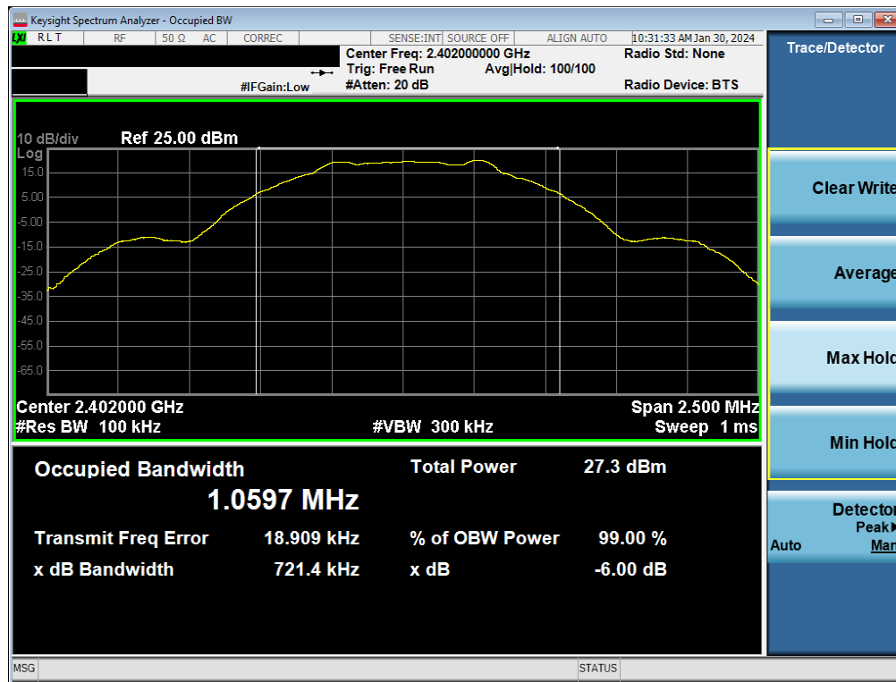
Plot 7-13. 6dB BW & 99% OBW Plot Antenna WF9 (Bluetooth (LE), 1Mbps, ePA – Ch. 0)
