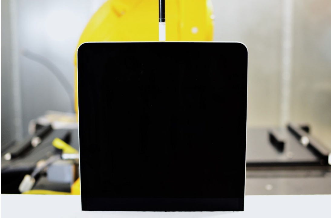
Near Field Power Density Test Setup Photo 16: Bottom Edge at 2mm – WF7/WF8/WF5B
