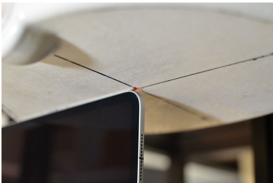
SAR Test Setup Photo 8: Left Edge at 0mm – WF7/WF9
