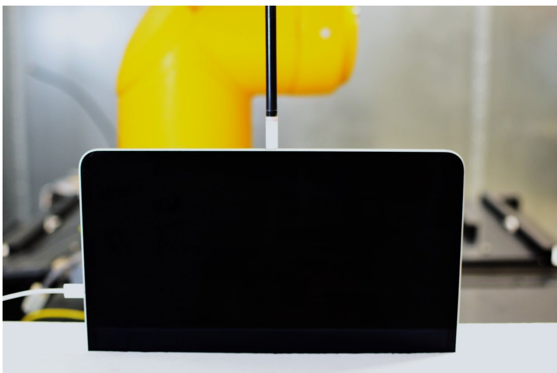
Near Field Power Density Test Setup Photo 19: Left Edge at 2mm – WF7/WF8/WF5B
