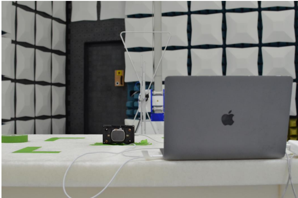
Figure 15: 30MHz-1GHz Test Setup (Rear View)
