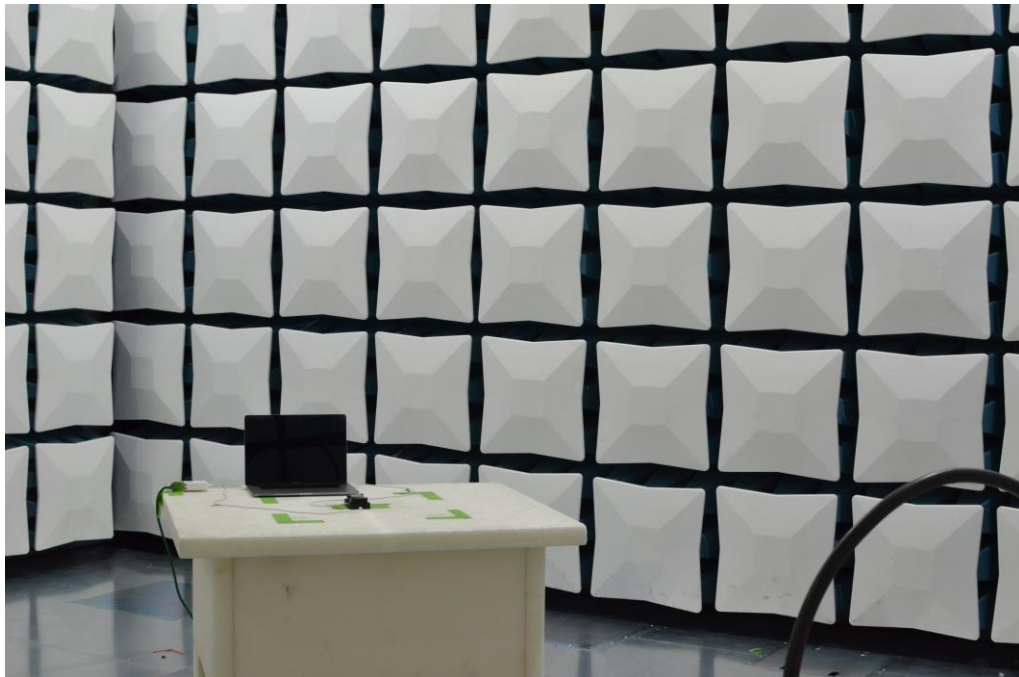
Figure 18: 9kHz-30MHz Test Setup (Front View)
