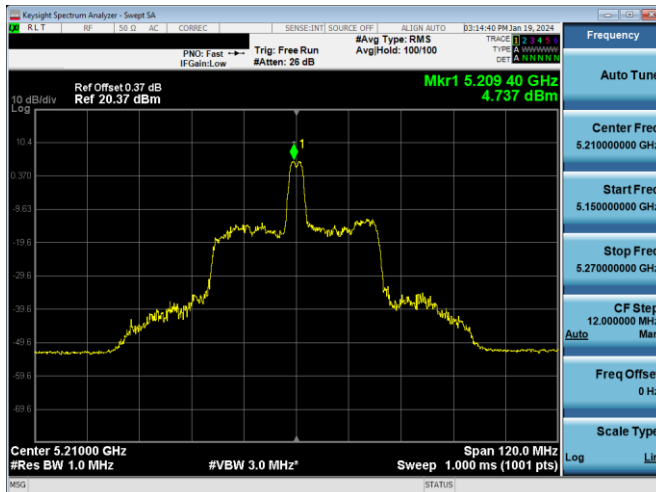
Plot 7-401. PSD CDD Antenna 3a (80MHz BW 11ax Index 18 - RU26 - Ch.42)
