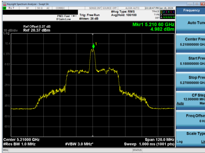
Plot 7-400. PSD CDD Antenna 3c (80MHz BW 11ax Index 18 - RU26 - Ch.42)
