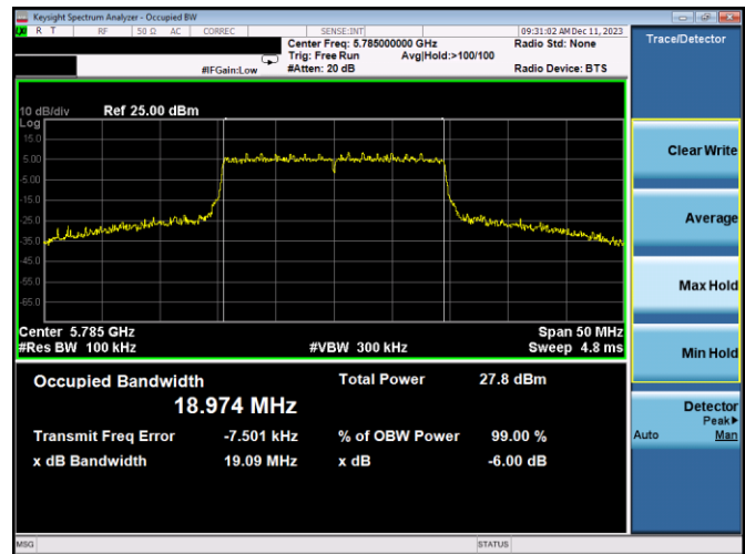
Plot 7-160. 6dB BW & 99% OBW Antenna 1b (20MHz BW 11ax – RU242 – Ch.157)
