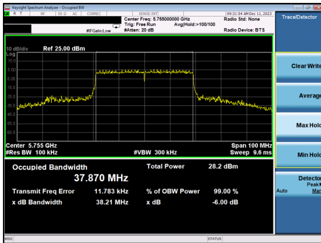
Plot 7-164. 6dB BW & 99% OBW Antenna 1b (40MHz BW 11ax – RU484 – Ch.151)
