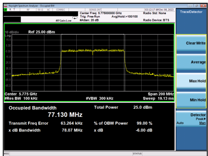
Plot 7-222. 6dB BW & 99% OBW Antenna 3a (80MHz BW 802.11ax(SU) – Ch. 155, MCS2)
