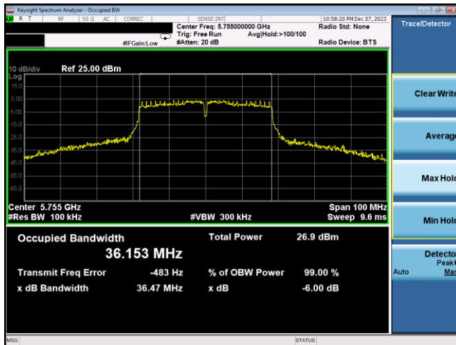
Plot 7-207. 6dB BW & 99% OBW Antenna 3c (40MHz BW 802.11n – Ch. 151, MCS4)
