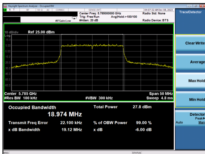
Plot 7-224. 6dB BW & 99% OBW Antenna 3a (20MHz BW 802.11ax(SU) – Ch. 157, MCS4)
