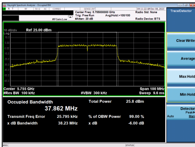
Plot 7-226. 6dB BW & 99% OBW Antenna 3a (40MHz BW 802.11ax(SU) – Ch. 151, MCS4)
