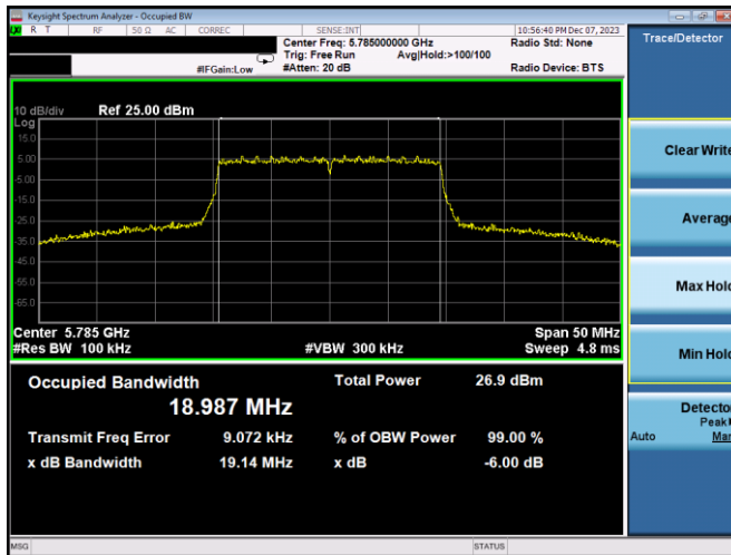
Plot 7-206. 6dB BW & 99% OBW Antenna 3c (20MHz BW 802.11ax(SU) – Ch. 157, MCS4)
