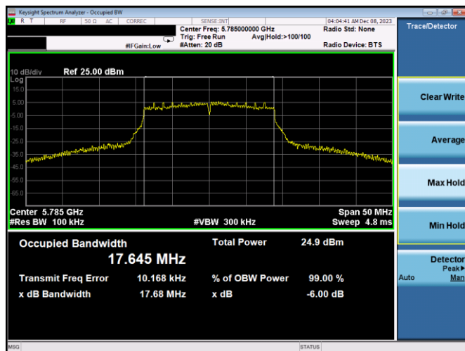
Plot 7-223. 6dB BW & 99% OBW Antenna 3a (20MHz BW 802.11n – Ch. 157, MCS4)
