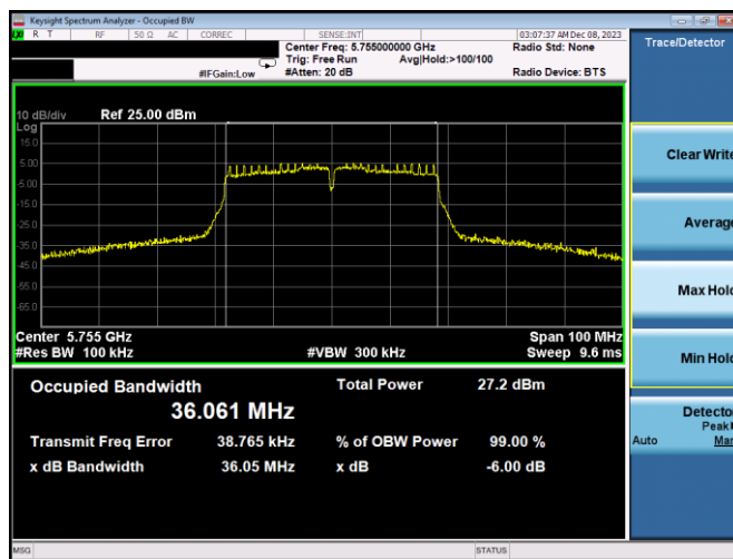
Plot 7-219. 6dB BW & 99% OBW Antenna 3a (40MHz BW 802.11n – Ch. 151, MCS2)
