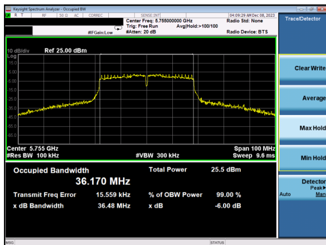
Plot 7-225. 6dB BW & 99% OBW Antenna 3a (40MHz BW 802.11n – Ch. 151, MCS4)
