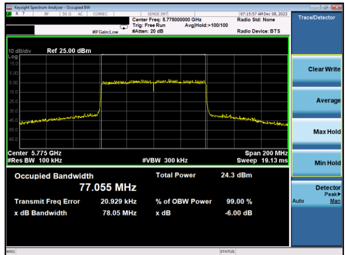
Plot 7-234. 6dB BW & 99% OBW Antenna 3a (80MHz BW 802.11ax(SU) – Ch. 155, MCS11)
