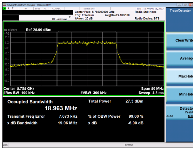
Plot 7-236. 6dB BW & 99% OBW Antenna 1b (20MHz BW 802.11ax(SU) – Ch. 157, MCS2)
