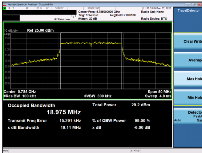
Plot 7-212. 6dB BW & 99% OBW Antenna 3c (20MHz BW 802.11ax(SU) – Ch. 157, MCS11)
