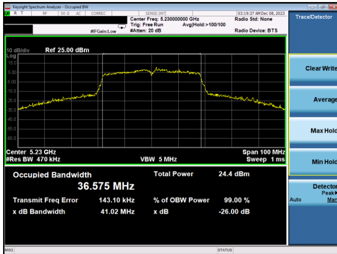
Plot 7-91. 26dB BW & 99% OBW Antenna 3a (40MHz BW 802.11n – Ch. 46, MCS4)
