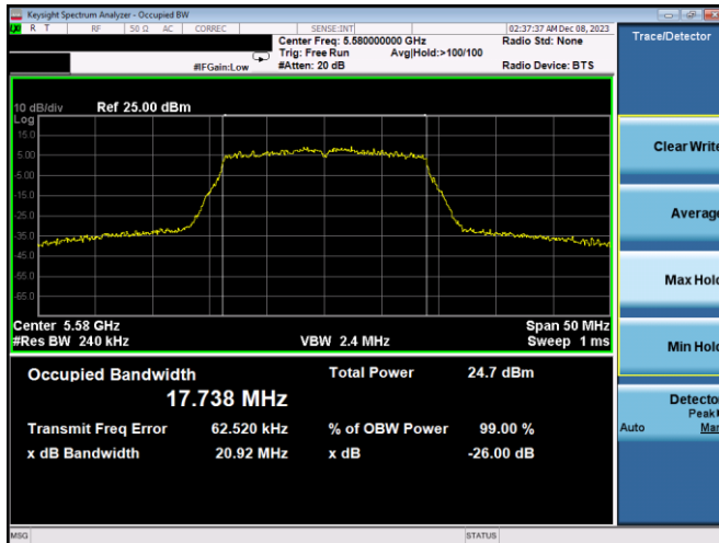
Plot 7-81. 26dB BW & 99% OBW Antenna 3a (20MHz BW 802.11n – Ch. 116, MCS2)
