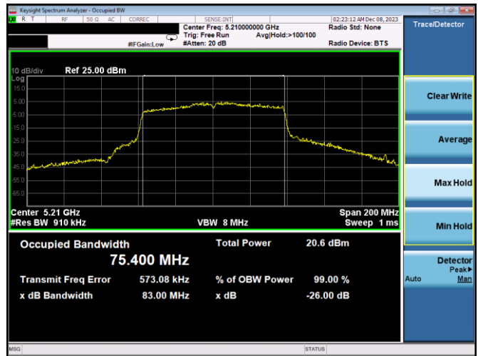
Plot 7-71. 26dB BW & 99% OBW Antenna 3a (80MHz BW 802.11ac – Ch. 42, MCS2)
