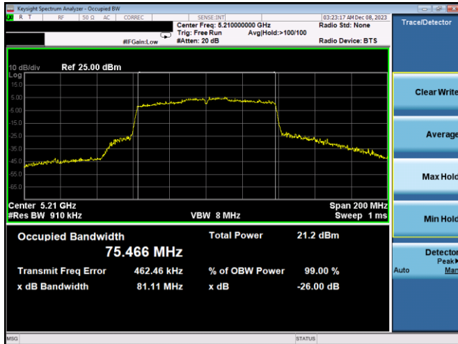
Plot 7-93. 26dB BW & 99% OBW Antenna 3a (80MHz BW 802.11ac – Ch. 42, MCS4)
