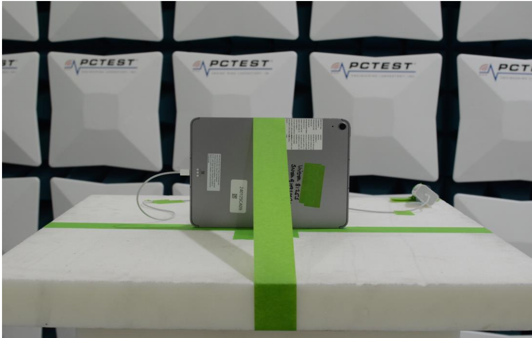
Figure 3: 1-18GHz Test Setup (Front View)
