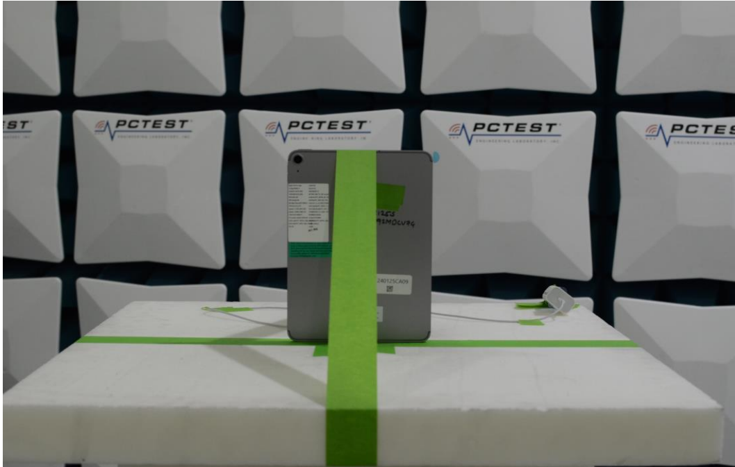
Figure 5: 1-18GHz Test Setup (Front View)
