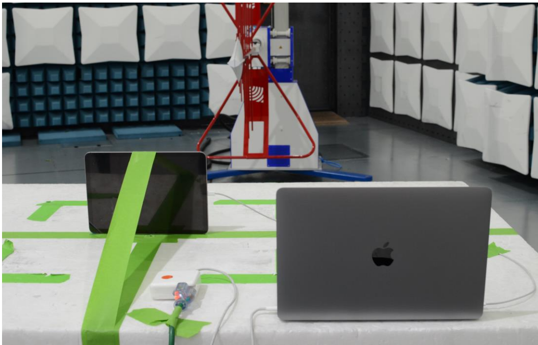
Figure 16: 30MHz-1GHz Test Setup (Rear View)
