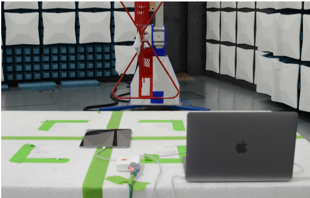
Figure 14: 30MHz-1GHz Test Setup (Rear View)
