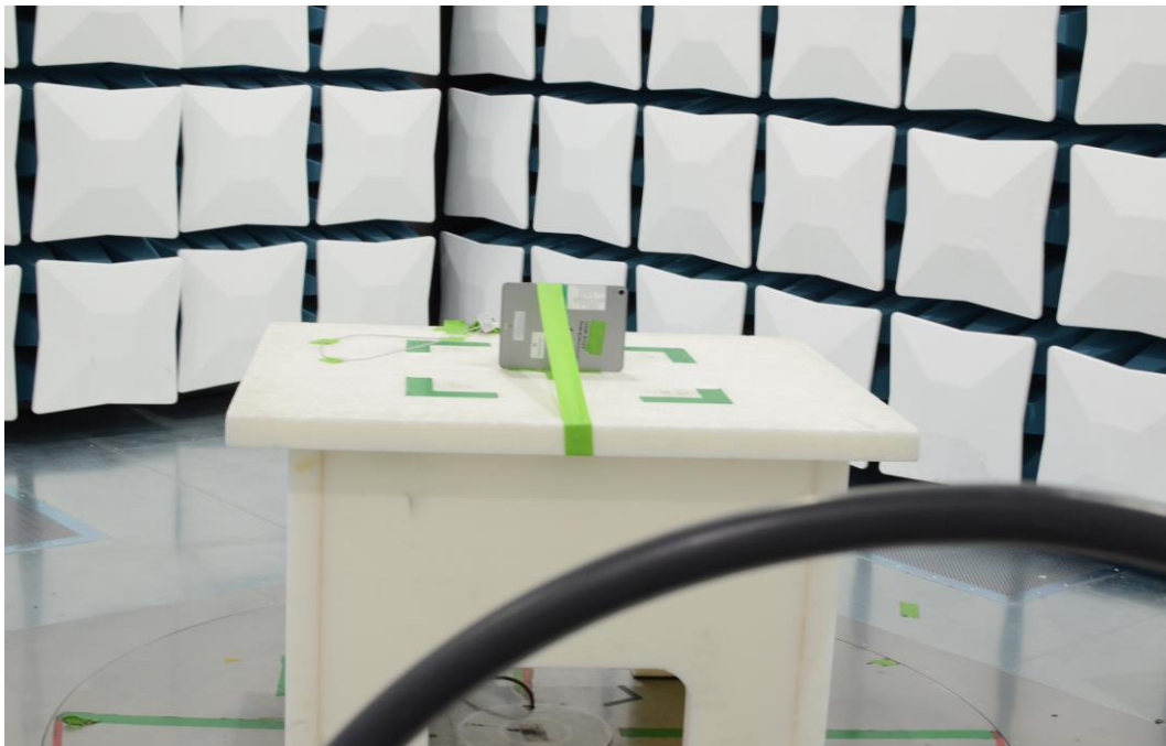
Figure 20: 9kHz-30MHz Test Setup (Front View)
