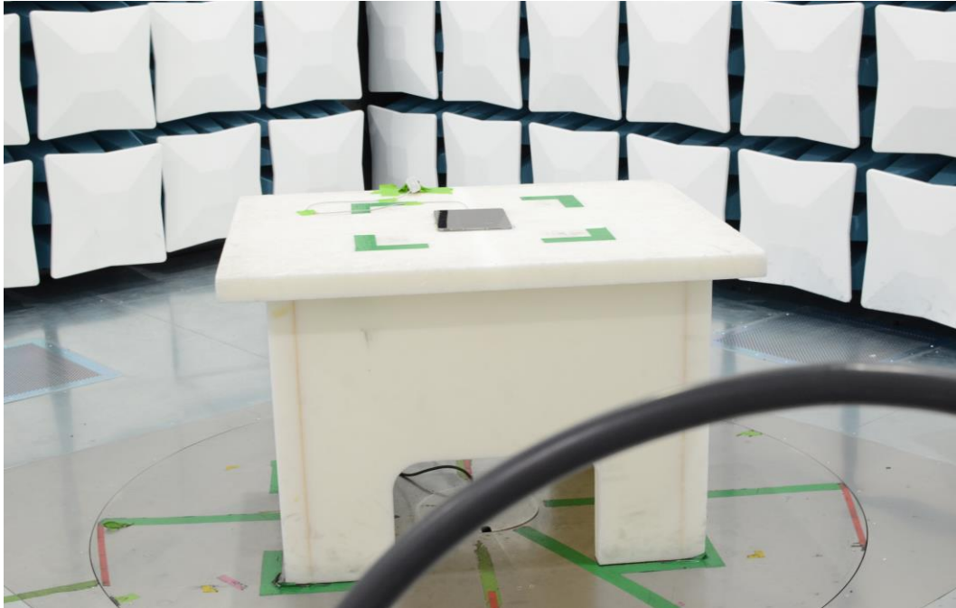
Figure 19: 9kHz-30MHz Test Setup (Front View)
