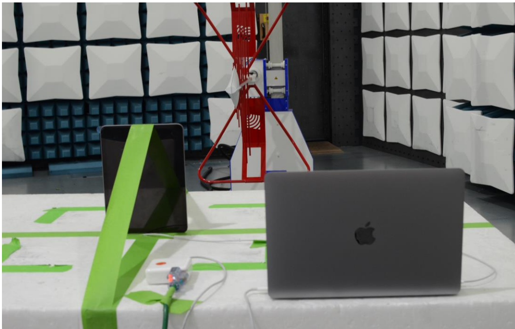
Figure 18: 30MHz-1GHz Test Setup (Rear View)
