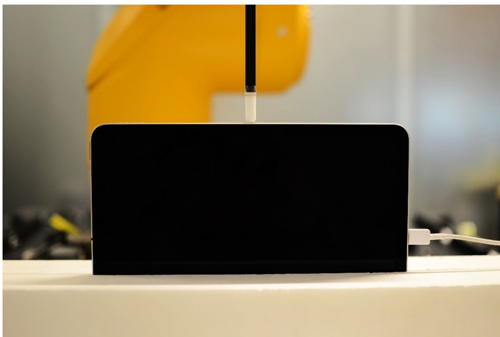
Near Field Power Density Test Setup Photo 10 – Right Edge at 2mm - WF8/7a
