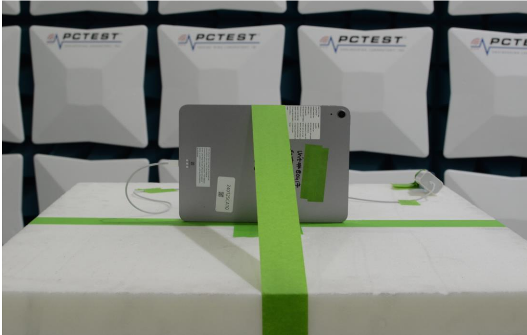
Figure 7: 1-18GHz Test Setup (Front View)
