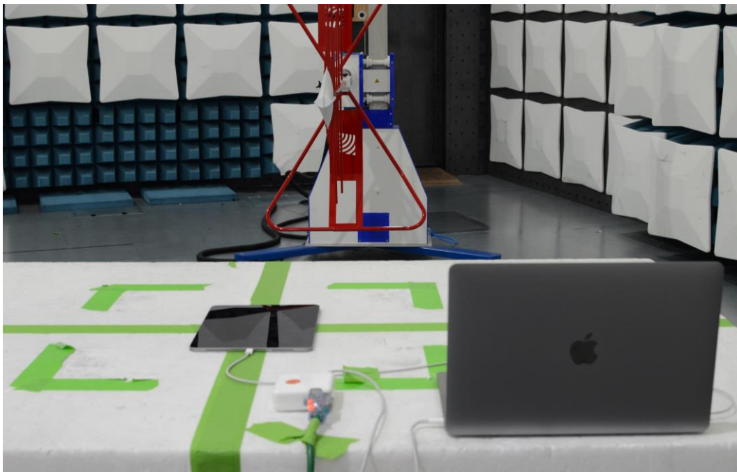
Figure 18: 30MHz-1GHz Test Setup (Rear View)
