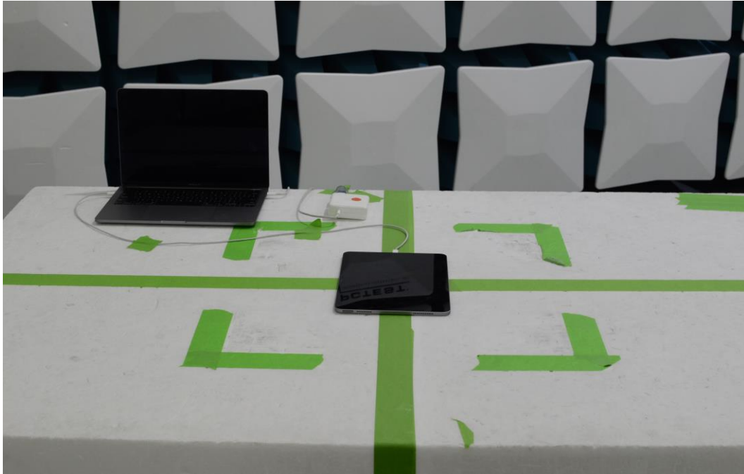
Figure 17: 30MHz-1GHz Test Setup (Front View)
