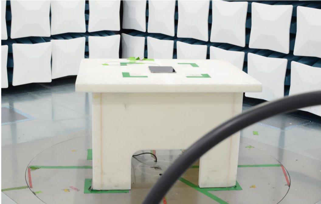
Figure 23: 9kHz-30MHz Test Setup (Front View)
