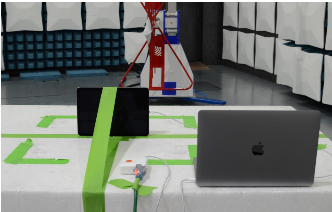
Figure 20: 30MHz-1GHz Test Setup (Rear View)
