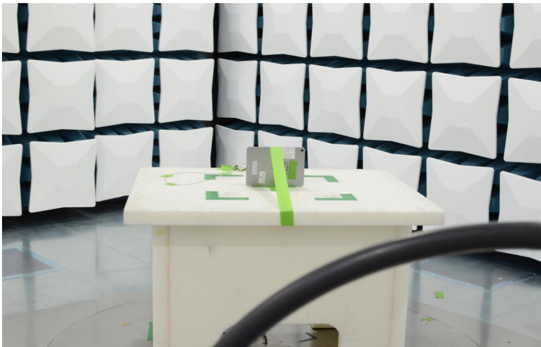
Figure 24: 9kHz-30MHz Test Setup (Front View)
