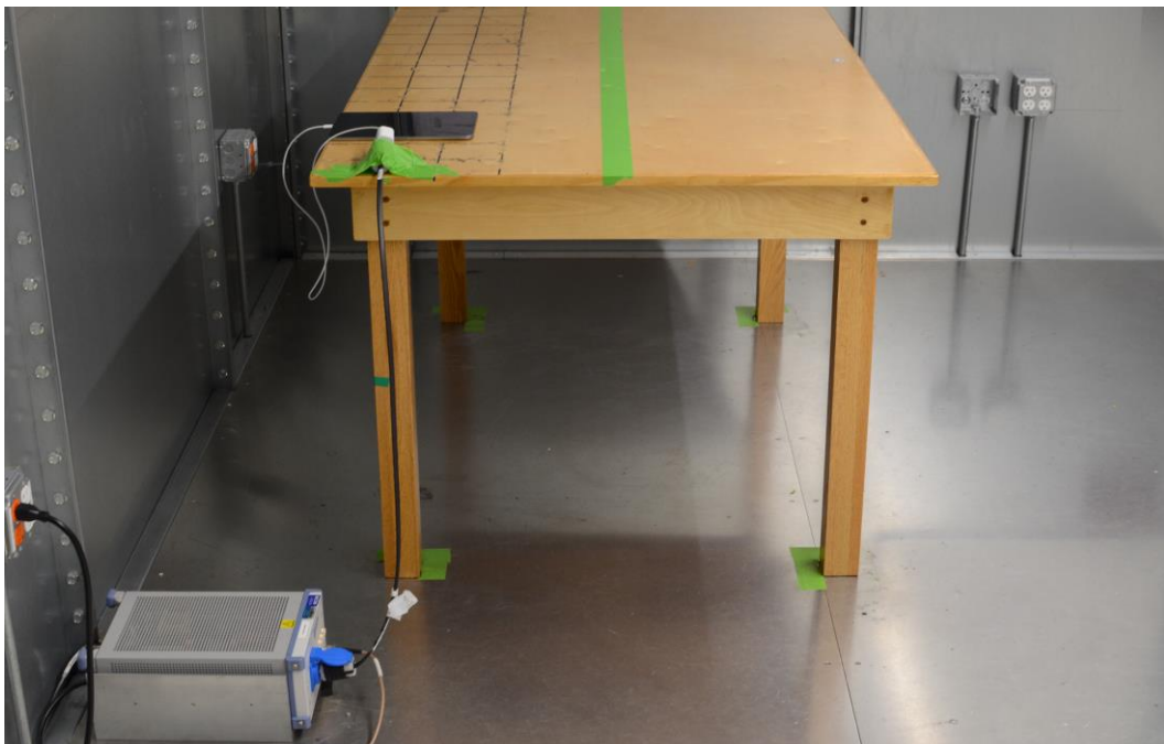
Figure 2: AC Line Conducted Emissions (Side View)
