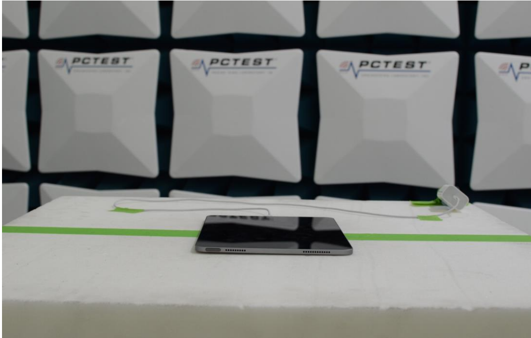
Figure 5: 1-18GHz Test Setup (Front View)
