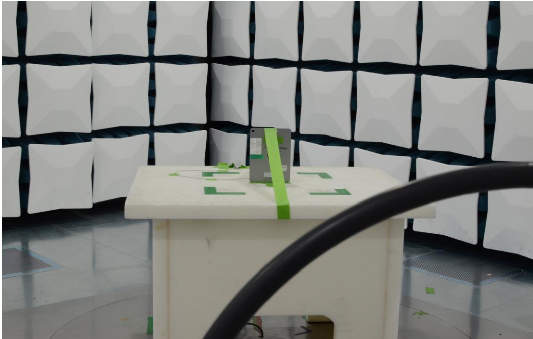
Figure 25: 9kHz-30MHz Test Setup (Front View)
