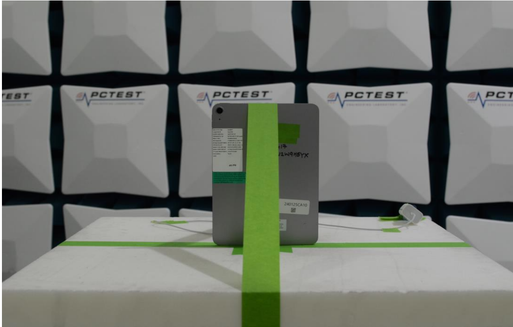
Figure 9: 1-18GHz Test Setup (Front View)
