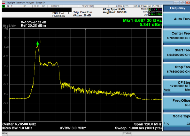
Plot 7-401. SP Power Spectral Density Plot CDD Diversity Antenna 5T (80MHz 802.11ax RU26 (UNII Band 7) – Ch. 151)
