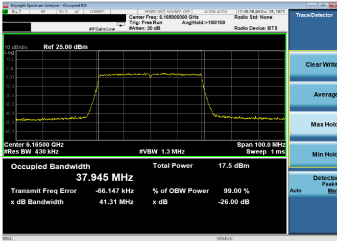
Plot 7-8. 26dB & 99% Bandwidth Plot Antenna 5T (40MHz 802.11ax RU484 (UNII Band 5) – Ch. 43)
