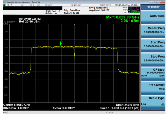
Plot 7-360. Power Spectral Density Plot Antenna 3b Standard Power (160MHz 802.11ax (UNII Band 7) – Ch. 143, MCS11)
