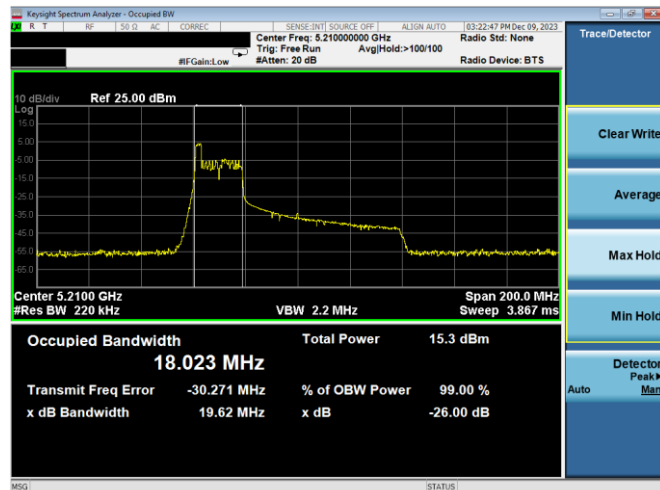
Plot 7-53. 26dB BW & 99% OBW Antenna WF2a (80MHz BW 11ax Index 0 – RU26 – Ch.42)
