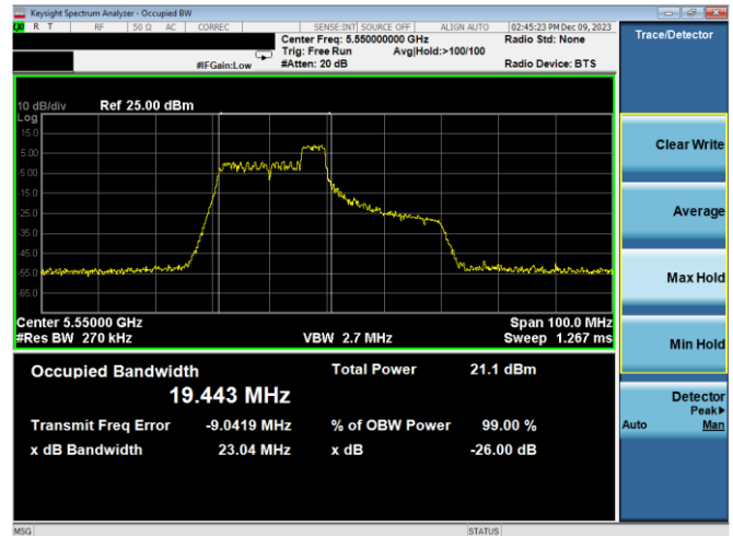
Plot 7-34. 26dB BW & 99% OBW Antenna WF7a (40MHz BW 11ax Index 40 – RU52 – Ch.110)
