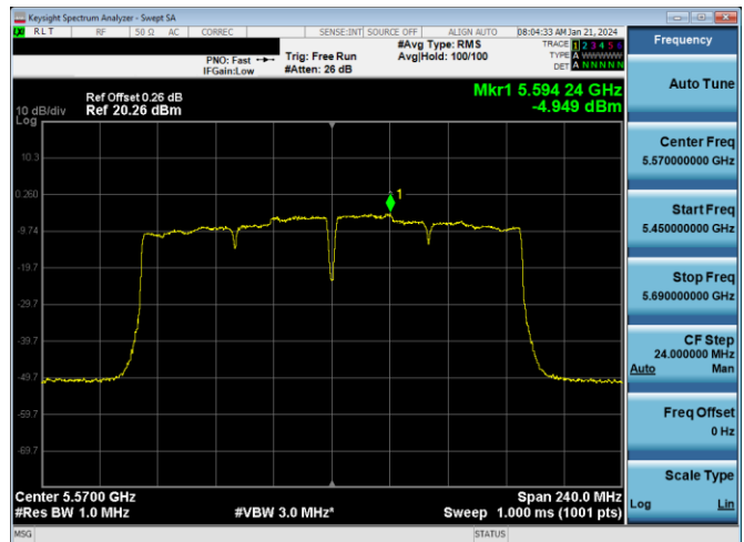
Plot 7-618. PSD CDD PRIMARY Antenna WF2a (160MHz BW 802.11ac – Ch. 114, MCS2)
