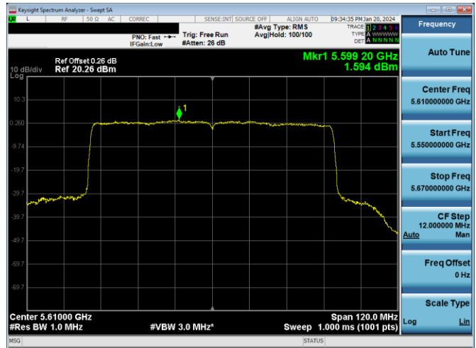
Plot 7-659. PSD CDD PRIMARY Antenna WF7a (80MHz BW 802.11ax(SU) – Ch. 122, MCS4)
