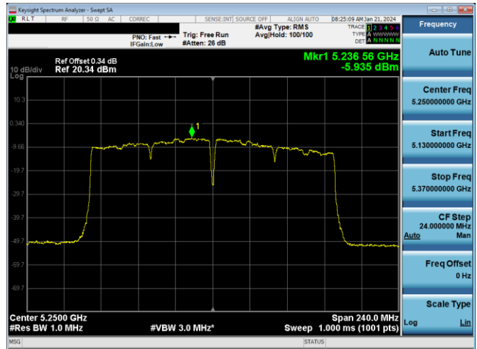
Plot 7-634. PSD CDD PRIMARY Antenna WF2a (160MHz BW 802.11ac – Ch. 50, MCS4)
