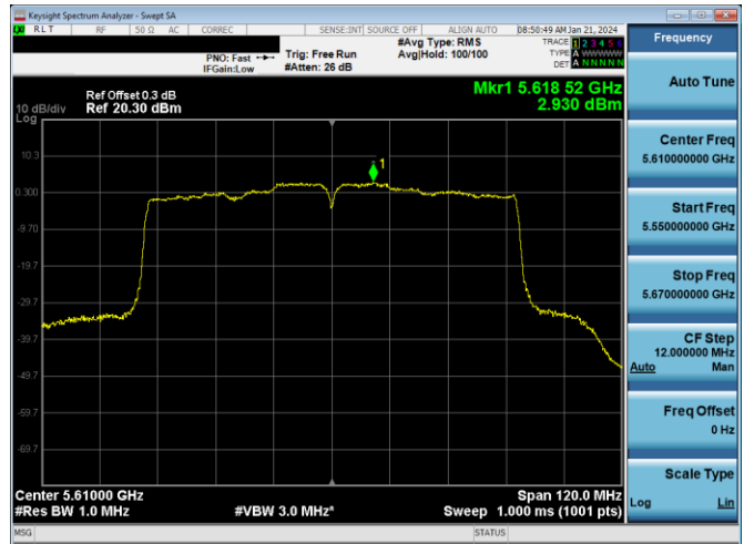
Plot 7-658. PSD CDD PRIMARY Antenna WF2a (80MHz BW 802.11ac – Ch. 122, MCS4)
