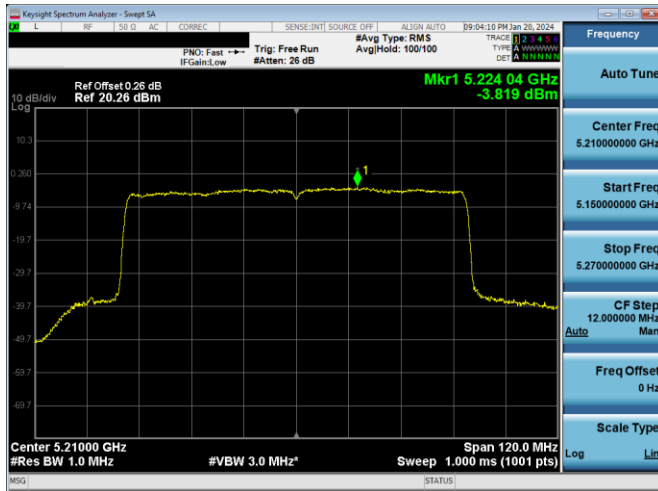
Plot 7-631. PSD CDD PRIMARY Antenna WF7a (80MHz BW 802.11ax(SU) – Ch. 42, MCS4)
