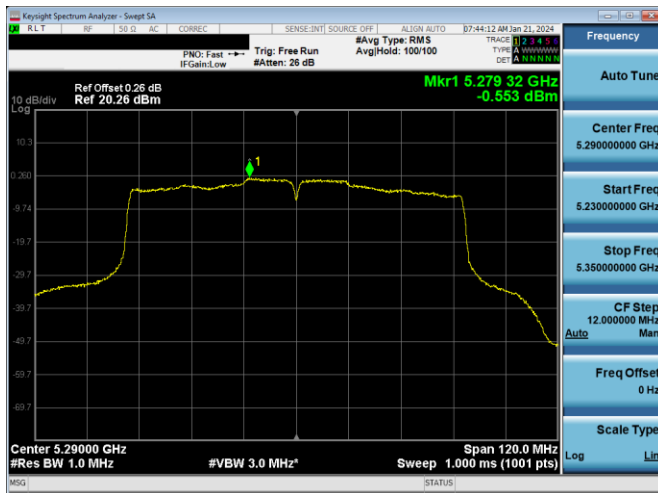
Plot 7-602. PSD CDD PRIMARY Antenna WF2a (80MHz BW 802.11ac - Ch. 58, MCS2)
