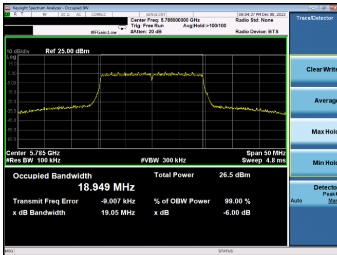
Plot 7-236. 6dB BW & 99% OBW Antenna WF2a (20MHz BW 802.11ax(SU) – Ch. 157, MCS2)
