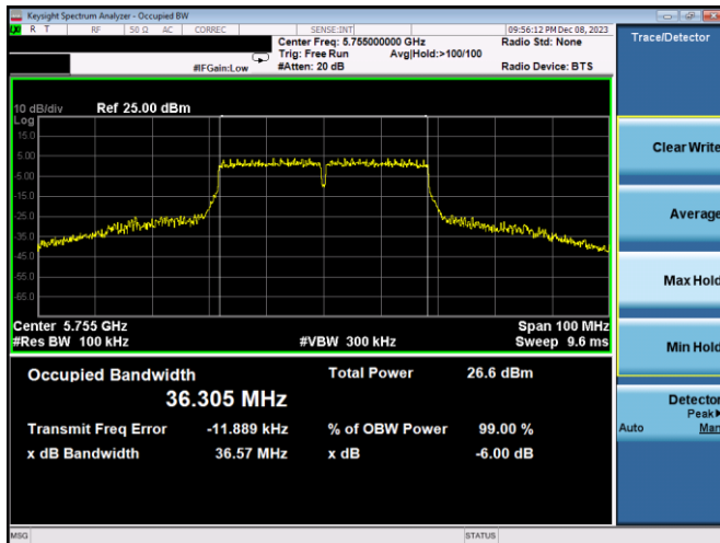
Plot 7-249. 6dB BW & 99% OBW Antenna WF2a (40MHz BW 802.11n – Ch. 151, MCS7)
