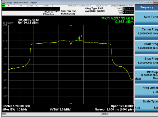
Plot 7-265. PSD Antenna WF7a (80MHz BW 802.11ac – Ch. 58, MCS2)
