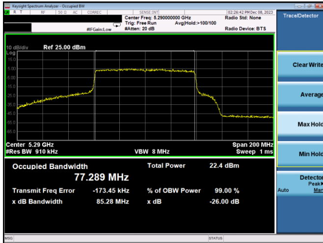
Plot 7-80. 26dB BW & 99% OBW Antenna WF7b (80MHz BW 802.11ax(SU) - Ch. 58, MCS2)
