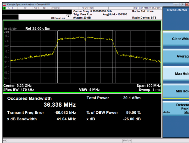
Plot 7-91. 26dB BW & 99% OBW Antenna WF7b (40MHz BW 802.11n – Ch. 46, MCS4)
