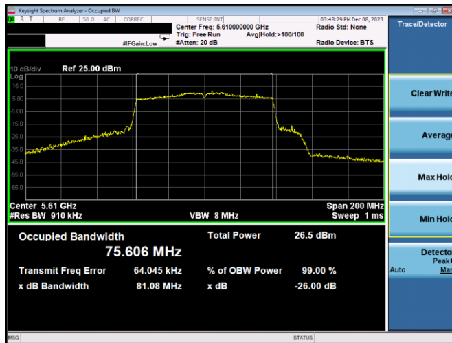
Plot 7-107. 26dB BW & 99% OBW Antenna WF7b (80MHz BW 802.11ac – Ch. 122, MCS4)
