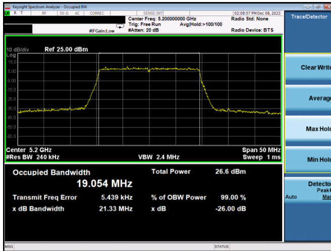
Plot 7-68. 26dB BW & 99% OBW Antenna WF7b (20MHz BW 802.11ax(SU) – Ch. 40, MCS2)
