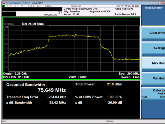
Plot 7-79. 26dB BW & 99% OBW Antenna WF7b (80MHz BW 802.11ac - Ch. 58, MCS2)
