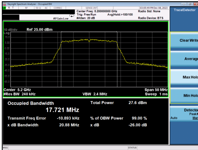
Plot 7-89. 26dB BW & 99% OBW Antenna WF7b (20MHz BW 802.11n – Ch. 40, MCS4)
