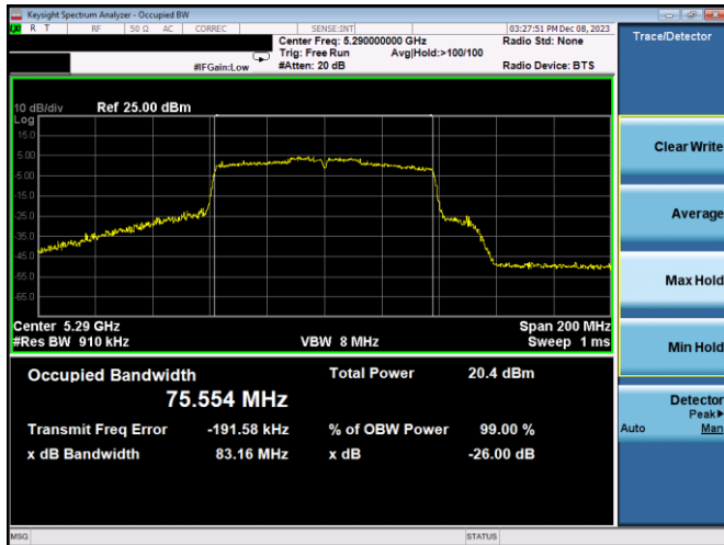
Plot 7-101. 26dB BW & 99% OBW Antenna WF7b (80MHz BW 802.11ac – Ch. 58, MCS4)
