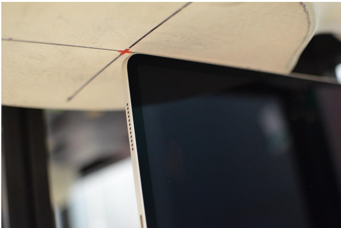
SAR Test Setup Photo 9: Left Edge at 0mm – WF2A/WF2b
