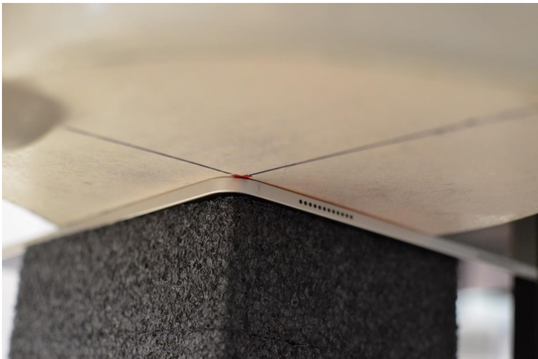
SAR Test Setup Photo 3: Back Side at 0mm – Ant WF7b
