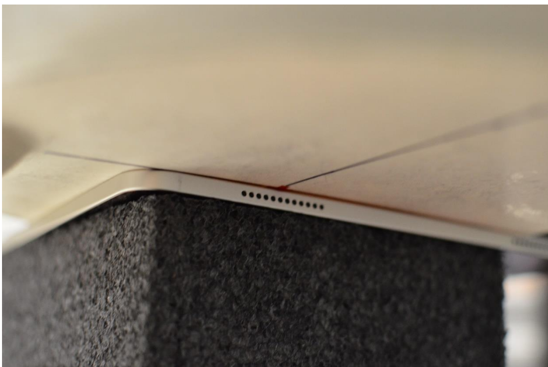
SAR Test Setup Photo 4: Back Side at 0mm – Ant WF7a
