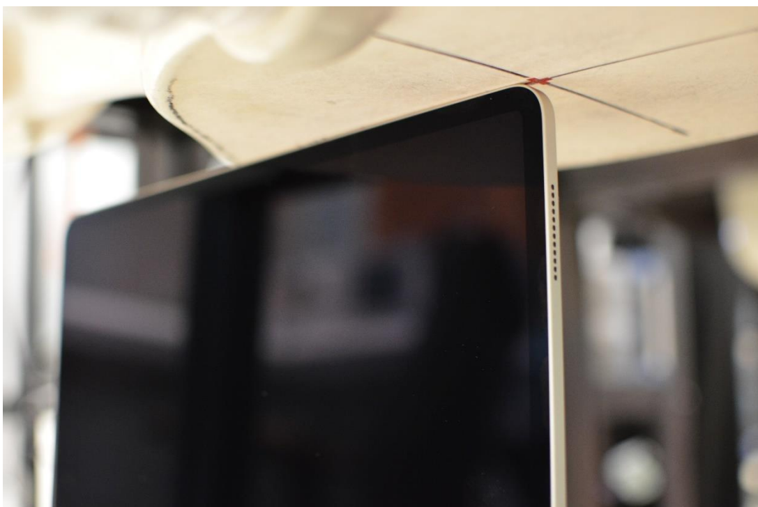
SAR Test Setup Photo 10: Left Edge at 0mm – WF7A/WF7b
