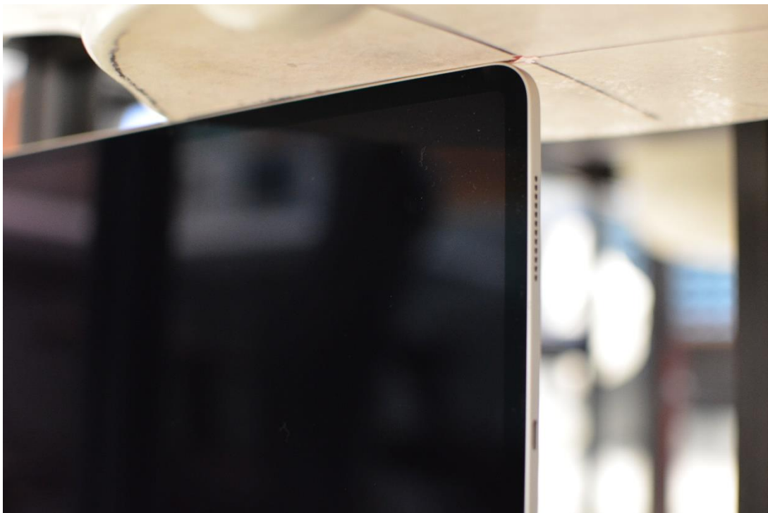
SAR Test Setup Photo 7: Right Edge at 0mm – WF2A/WF2b
