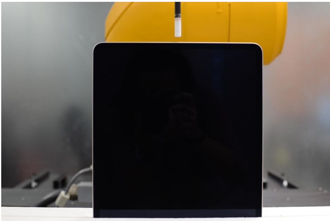
Near Field Power Density Test Setup Photo 19: Bottom Edge at 9.95mm – WF2a
