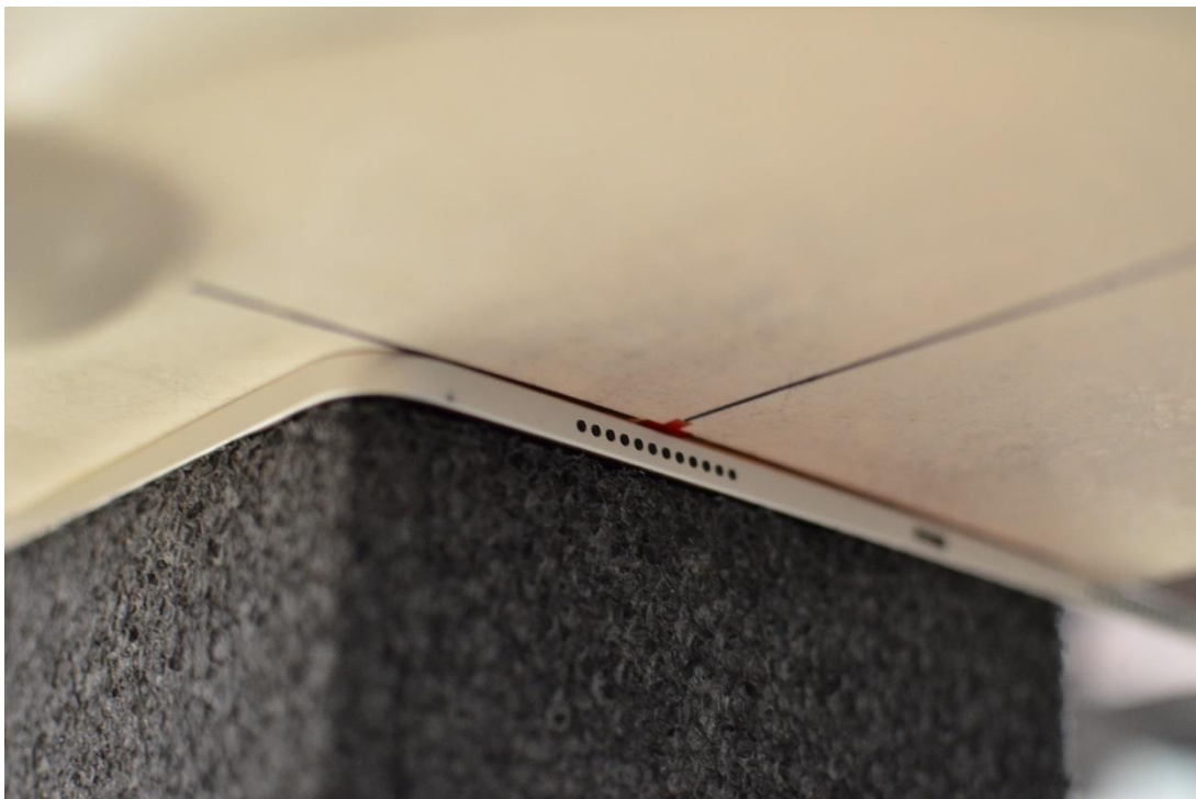
SAR Test Setup Photo 1: Back Side at 0mm – Ant WF2A
