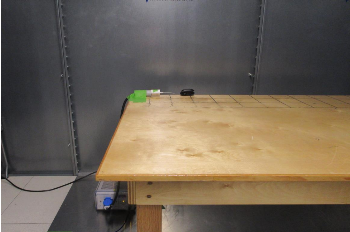
Figure 13: AC Line Test Setup (Front View)
