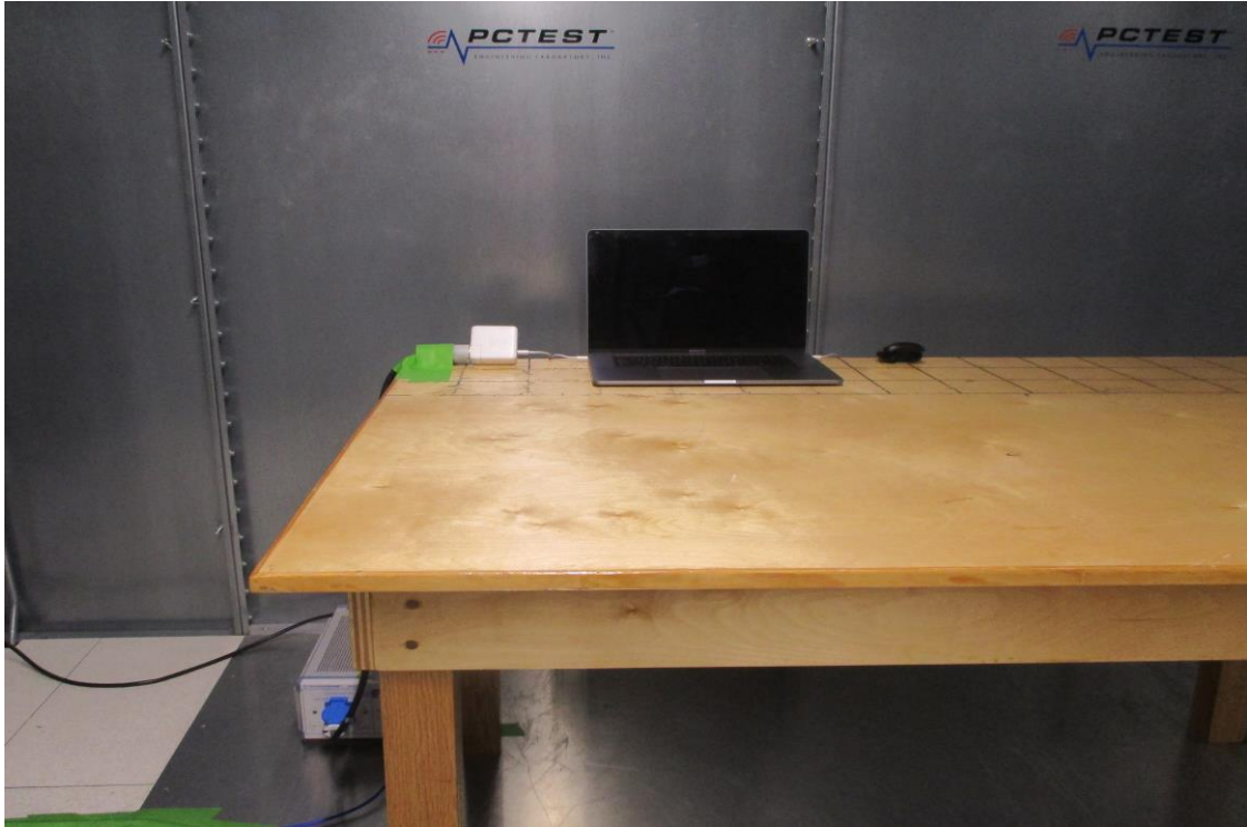
Figure 15: AC Line Test Setup (Front View)
