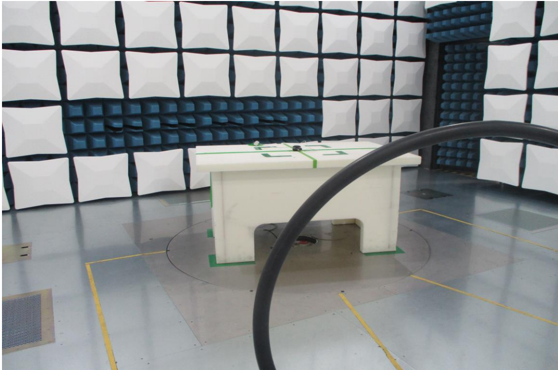
Figure 17: 9kHz-30MHz Test Setup (Front View)
