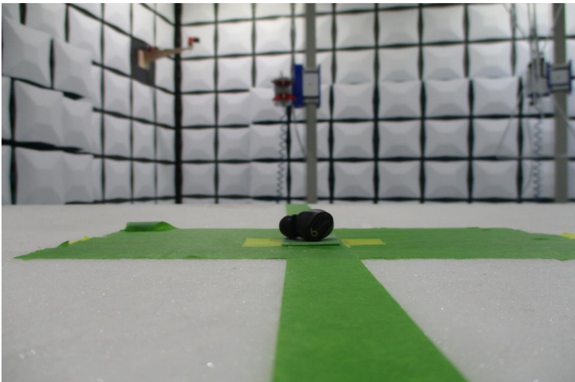
Figure 6: 1-18GHz Test Setup (Rear View)
