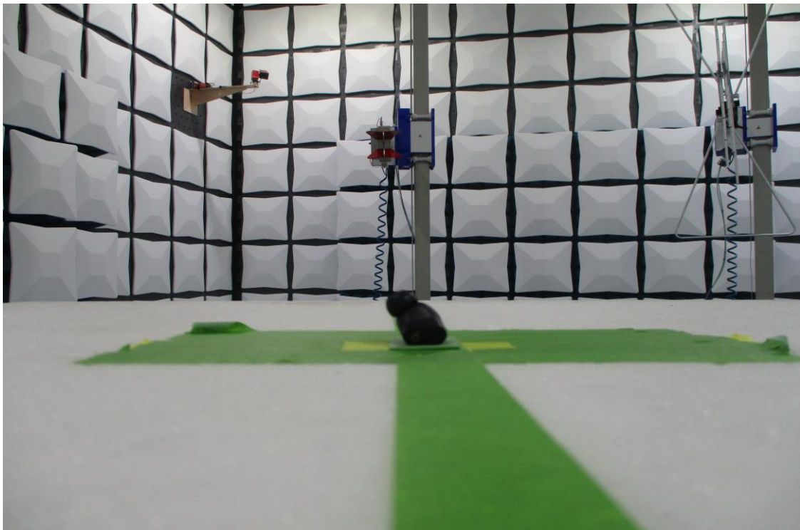
Figure 4: 1-18GHz Test Setup (Rear View)
